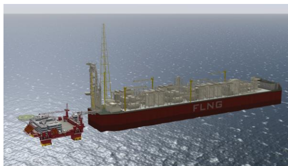
Figure 6. FLNG and ASV within Full mission Simulator (ASV gangway connected at stern) rotation point at forward turret ~480m forward of ASV
