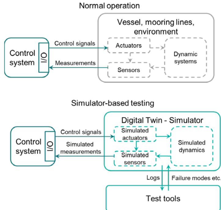
Figure 5: Simulator-based testing concept
