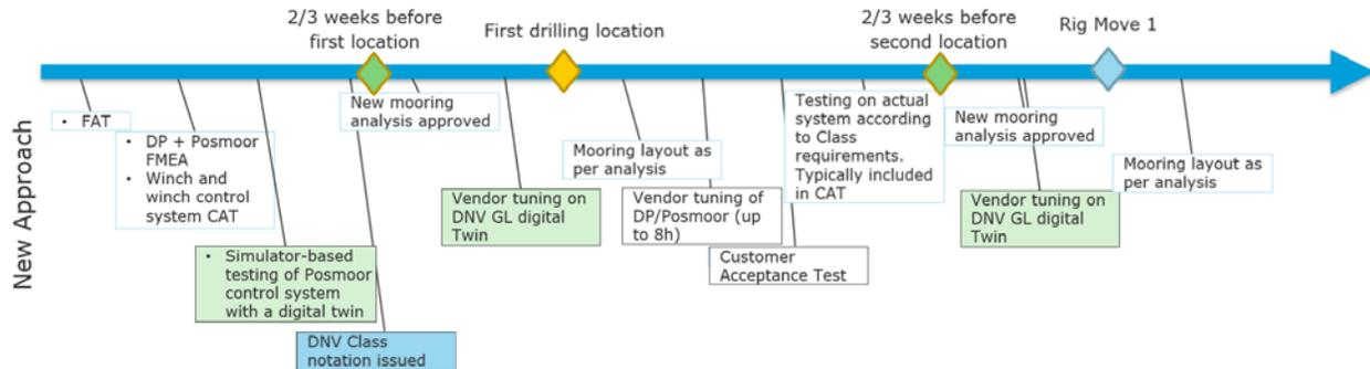
Figure 7: New DNV GL approach for POSMOOR-ATA
