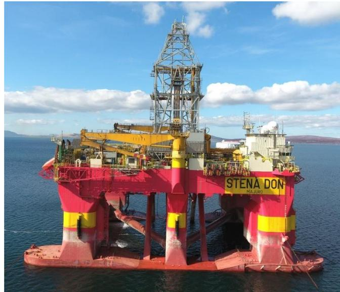
The Stena don is a DP 3 Classed 4<sup>th</sup> generation semi-Submersible drilling rig designed for mid water drilling, completion and intervention work by Kvaerner Maritime. It is a CS-30 design type and was built by Kvaerner Warnow Werft GmbH Germany and delivered in 2001.
