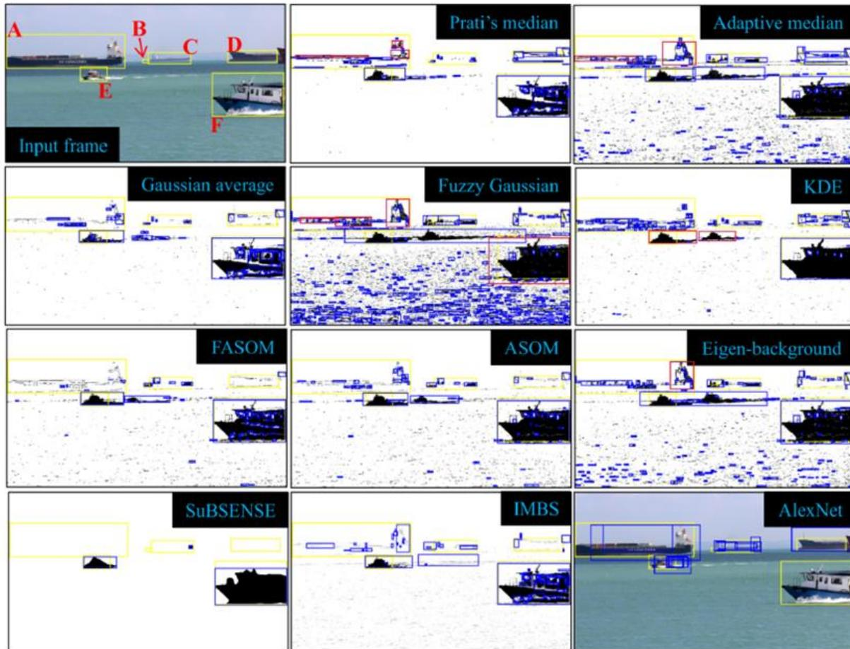
Figure 5: Dilip K. Prasad et al: Conventional vs. Machine Learning (AlexNet) picture recognition
