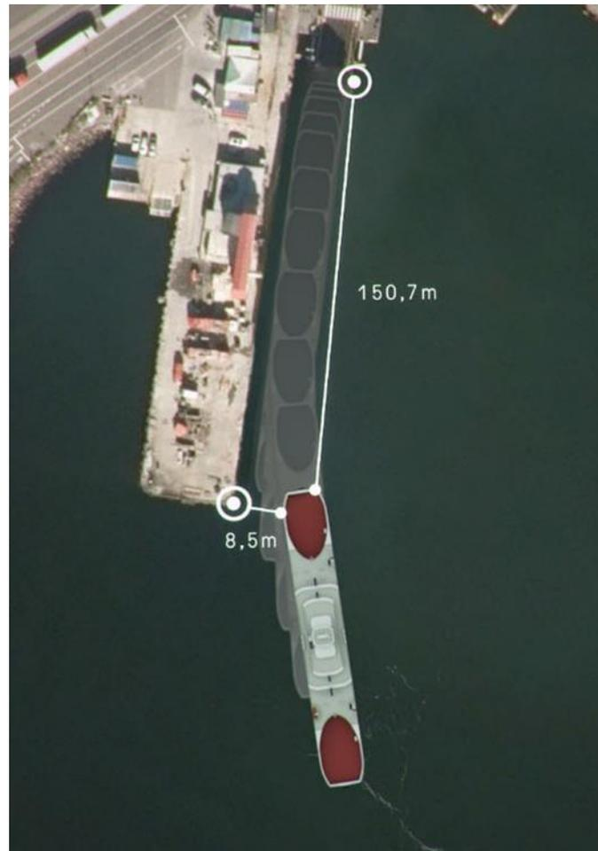
*Figure 6: Automated docking by sensor fusion and human supervision*
