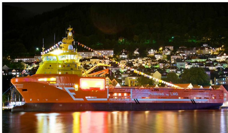
Figure 7 Viking Princess 511kWh – 1600kW – Spinning Reserve, Peak Shaving & Load Levelling (Start-Stop)
