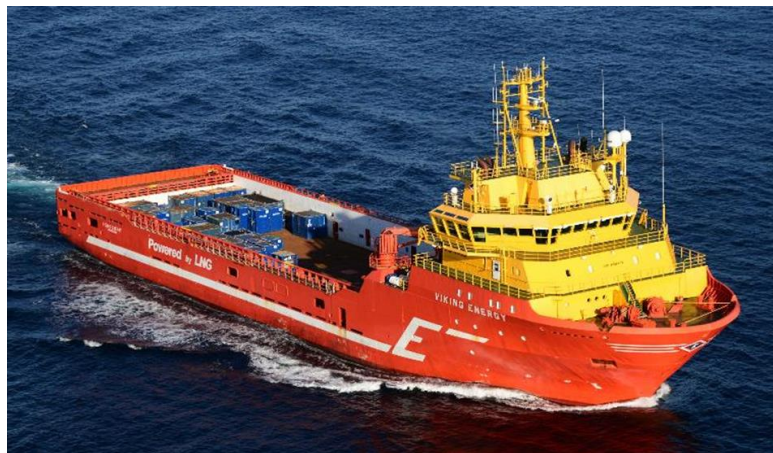
Figure 6 Viking Energy 652kWh – 1600kW – Spinning Reserve, Peak Shaving & Load Levelling (Start-Stop)
