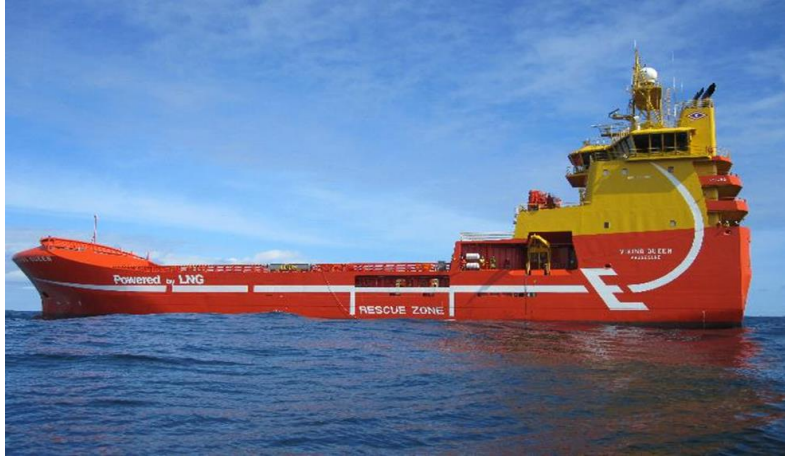
Figure 5 Viking Queen 652kWh – 1600kW – Peak Shaving & Load Leveling (Start-Stop)
