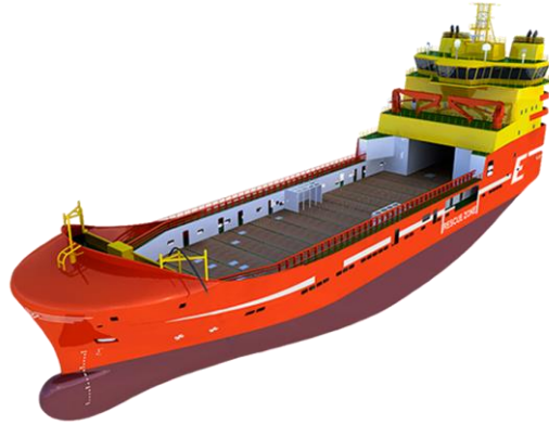
Figure 4 Viking Lady 442kWh – 900kW – Peak Shaving (& various test modes)
