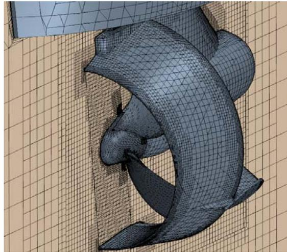
Figure 4: "Trimmer" Mesh in CCM+ on Azipod DZ1400P
