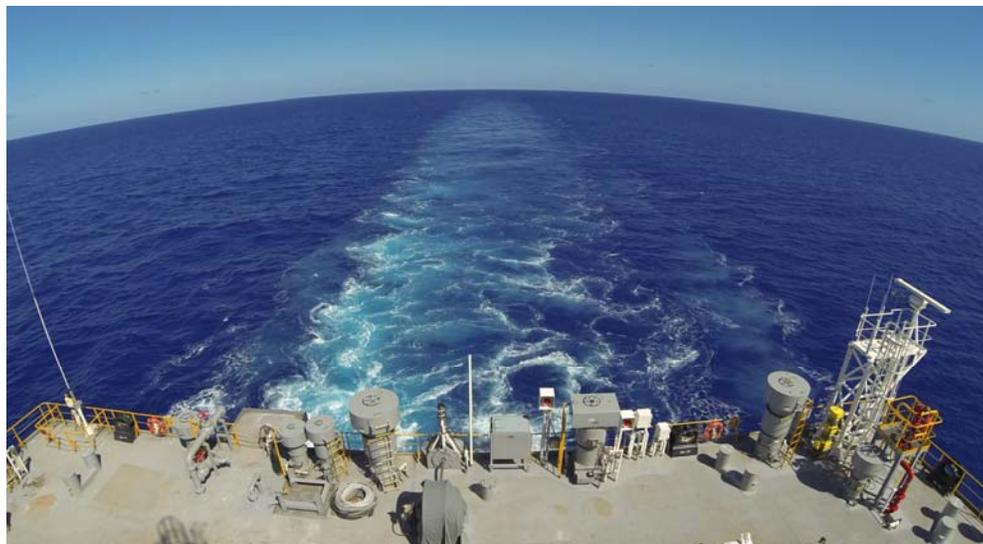
**Figure 3: Wake of *Ocean Blackhawk* Transiting Indian Ocean at ~12 knots, 70% power, 7 degree down-angle thrusters**
