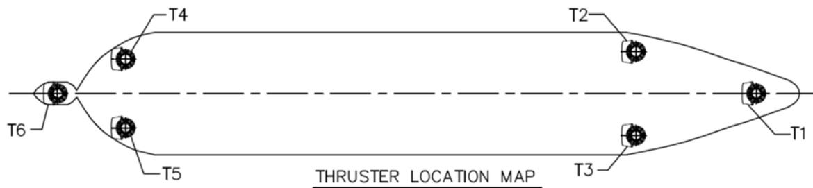
**Figure 6: Diamond Offshore Blackships Thruster Configuration**
