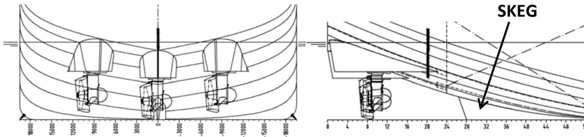
Figure 11: Floating Factory Aft Lines
