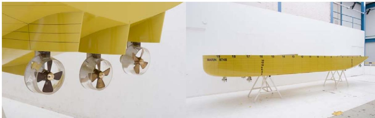
Figure 2: MARIN Tow-Tank Test Model (1:28.93 scale) with thrusters.
