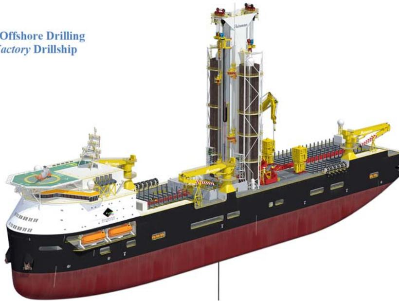
One of the central elements of the FF design is improved station-keeping efficiency, both to increase drilling up-time, and to reduce fuel consumption. To that end, we specified azimuthing thrusters with:
