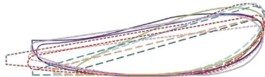
A pre design was carried out and tested in model scale. This verified good correspondence between the CFD results and the measured values in the towing tank. The free-running curve of the pre-design already promises a comparable bollard pull and an obvious improvement towards higher advanced ratios.
