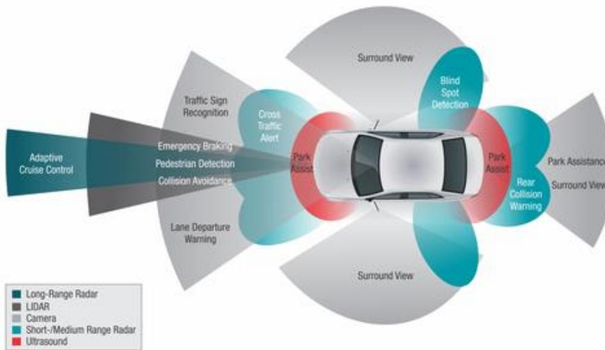
Figure 5: Sensors and sensor integration in a modern car
