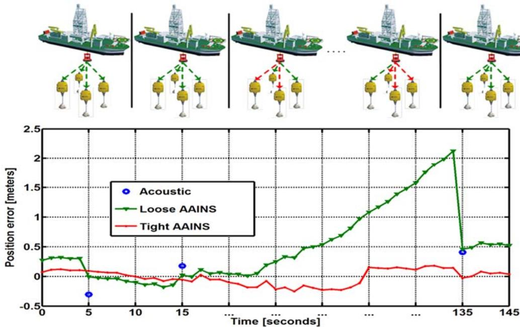
Figure 2 : Fault ride through advantage of tightly coupled
