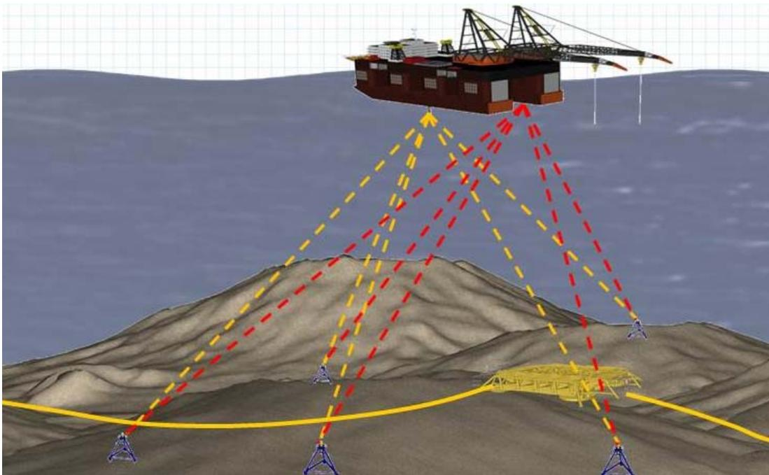
Figure 8 : A dual independent acoustic system sharing a seabed array with Multi-User transponders
