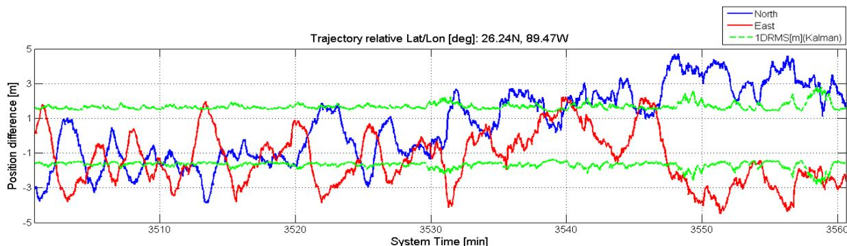
**Figure 4: Single transponder loosely coupled, 3000m water depth**
