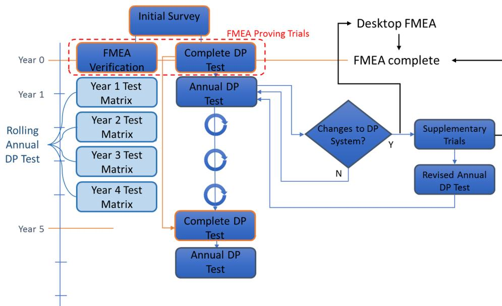
Figure 1 Evolution of DP Trials Throughout Vessel Lifetime
