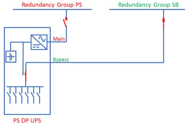
Figure 3 UPS in Bypass Configuration
