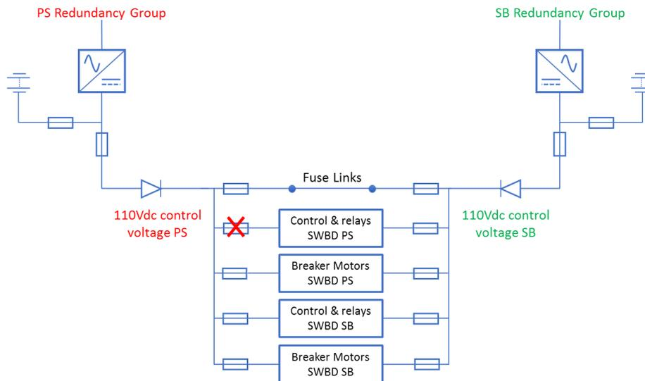
Figure 4 Cross Connections in 110Vdc Switchboard Control Voltages
