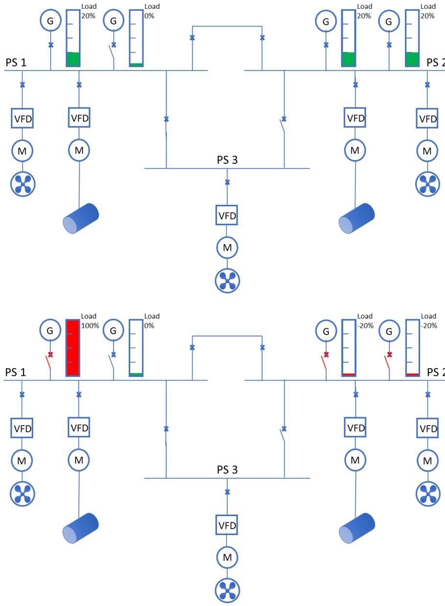
Figure 5 Closed Bus System Testing
