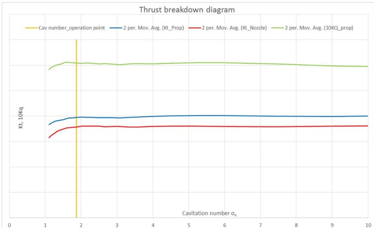
Figure 2. Thrust breakdown diagram for Bollard pull conditions. Yellow line presents the operating point of vessel with 100% Shaft power. The cavitation test was done with 1900kW.
