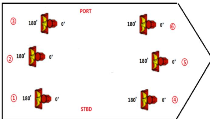
Figure 1 – Thruster Configuration
