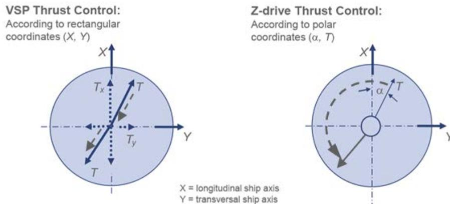
**Fig. 2 Thrust control principles of VSP and Z-drive Thrusters**
