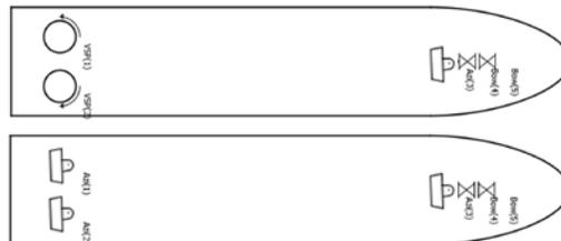
Fig. 4 thruster arrangement of the two examined variations
