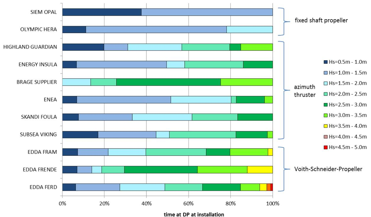
**Fig.13 Percentage of DP time at the platform during different significant wave heights**
