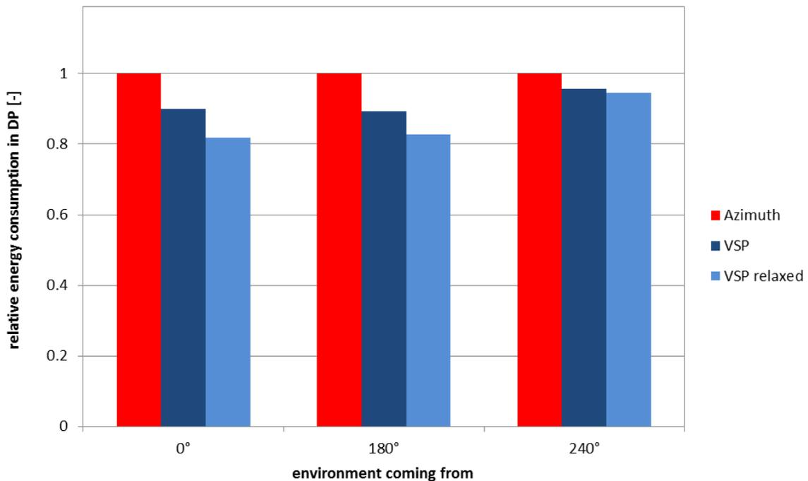
**Fig. 8 relative energy consumption of all thrusters during DP**
