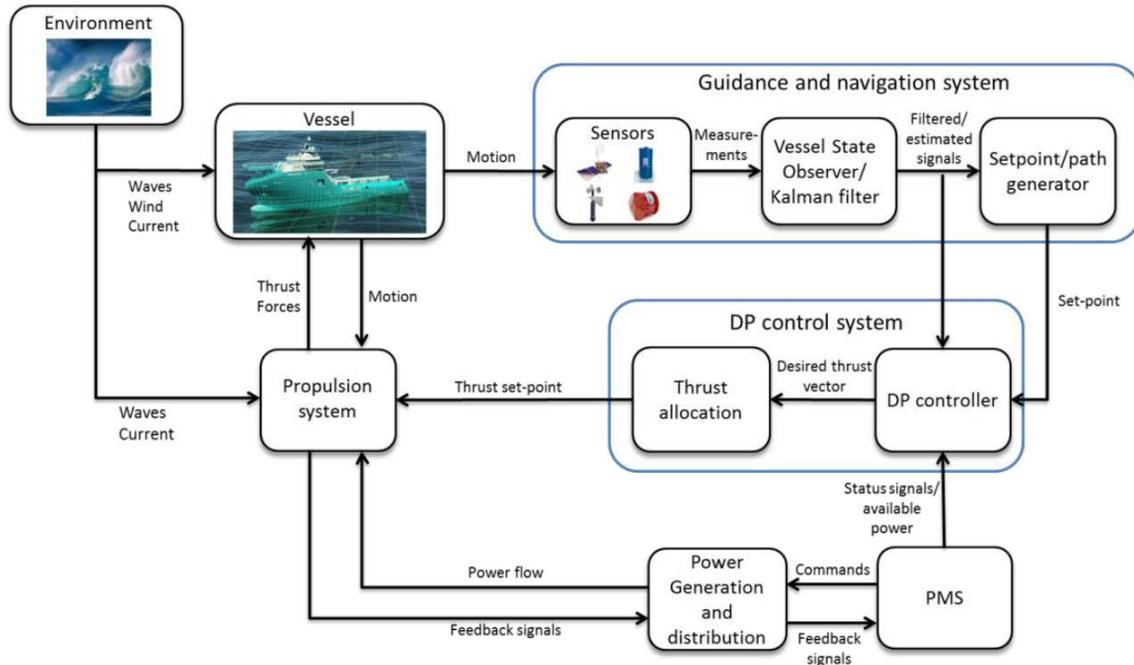
Fig. 3 DNV-GL Closed loop time-domain vessel simulator (figure taken from [1])
