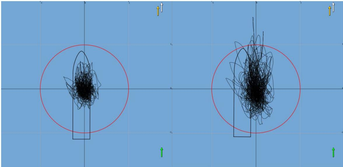
**Fig. 7 vessel footprint for stern on weather (VSP left, Azimuth right, wind speed 18m/s, red circle indicates acceptance limit of R=1m)**
