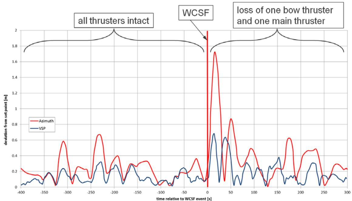
**Fig. 9 deviation from set point at WCSF conditions**
