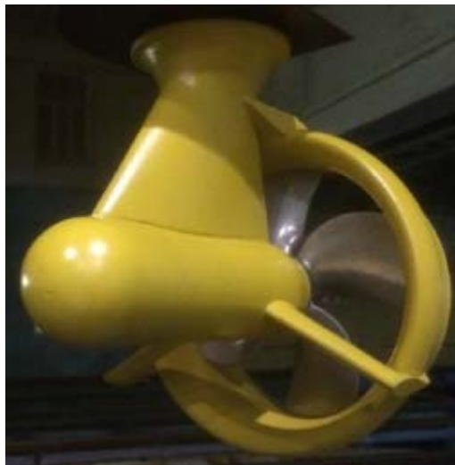
Azipod DZ open water test model.
