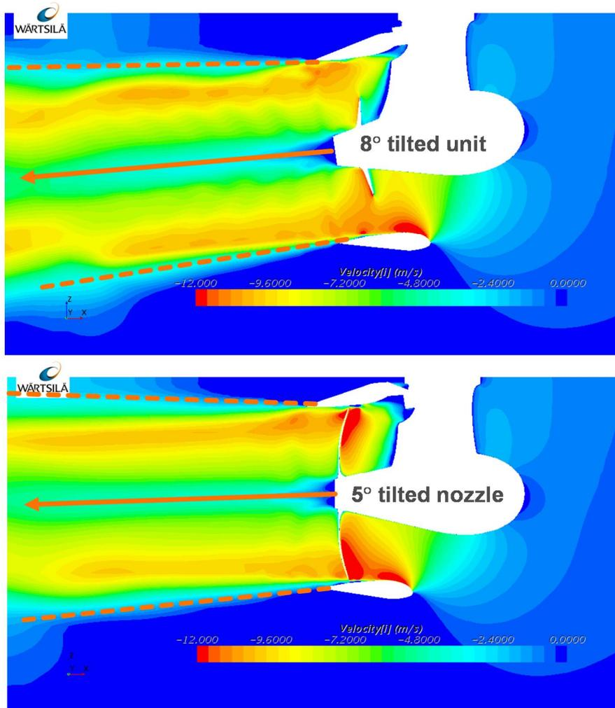
Figure 5: comparison of calculated wake of 8° tilted shaft and 5° tilted nozzle configuration
