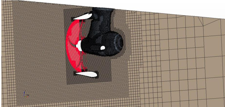
Figure 2: cross-sectional view of the mesh for the CFD simulations
