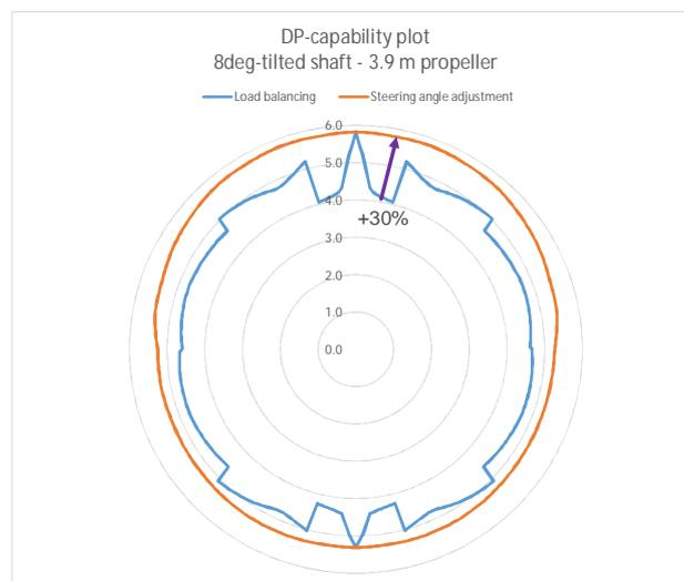
Figure 9: comparison of thrust allocation algorithms
