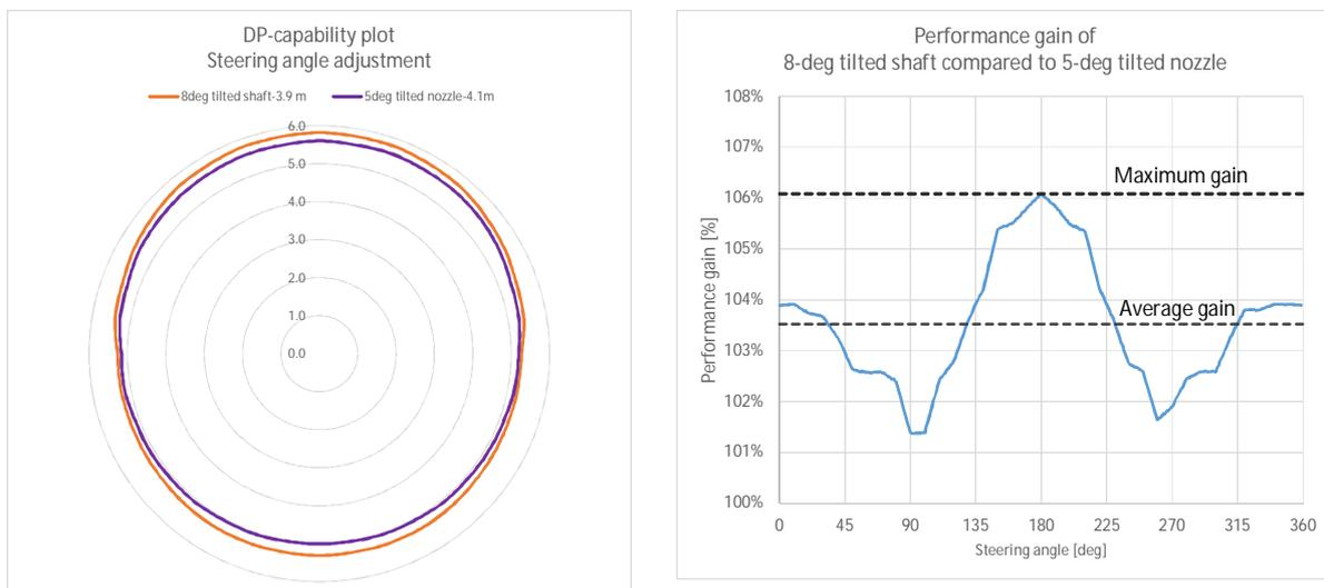
Figure 8: DP-capability comparison between 8° tilted shaft and 5° tilted nozzle configuration for 6 thrusters @ 5500 kW
