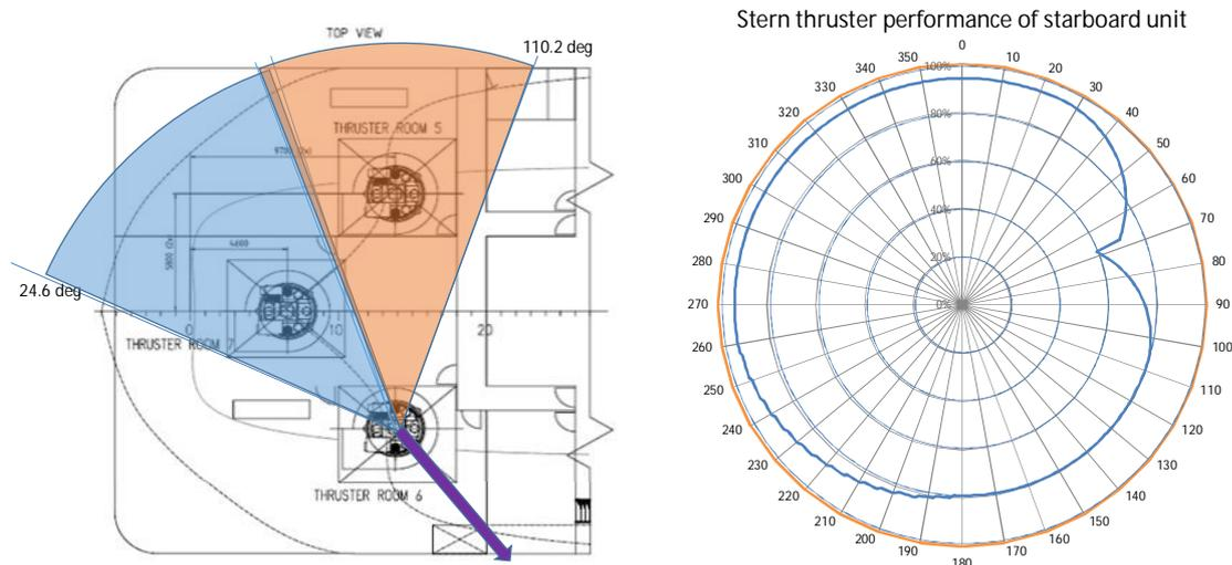
Figure 10: impact of two overlapping forbidden zones on thruster DP-capability
