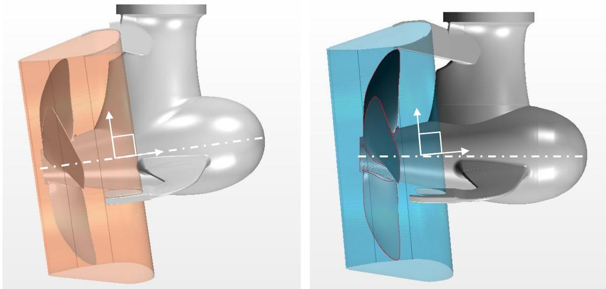
Figure 1: geometries of Wärtsilä WST-thruster with 8° tilted shaft and reference thruster unit with 5° tilted nozzle
