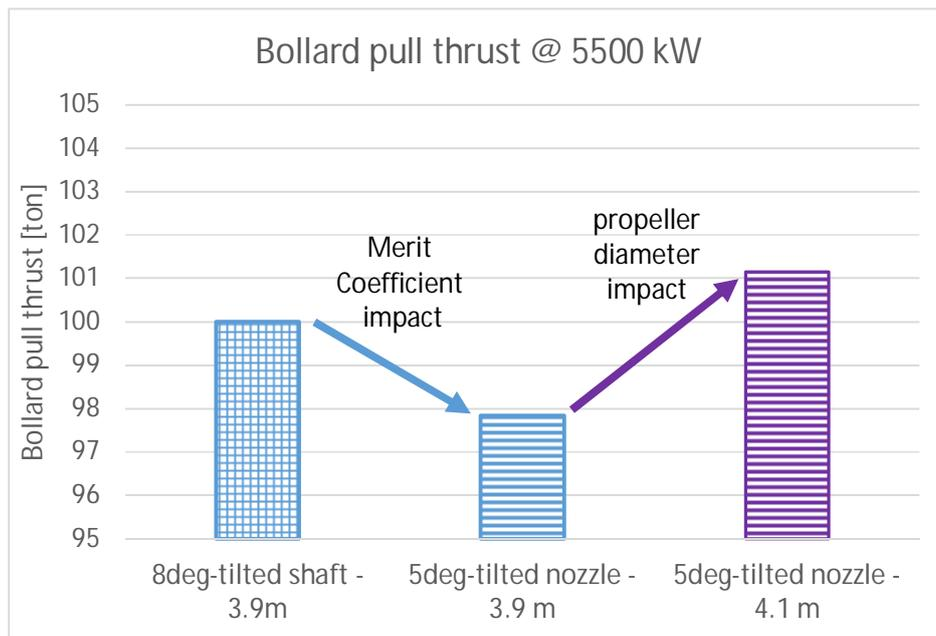
Figure 4: thruster bollard pull @ 5500 kW
