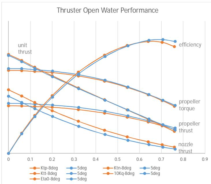
Figure 3: thruster open water performance for 8° tilted shaft unit and 5° tilted nozzle
