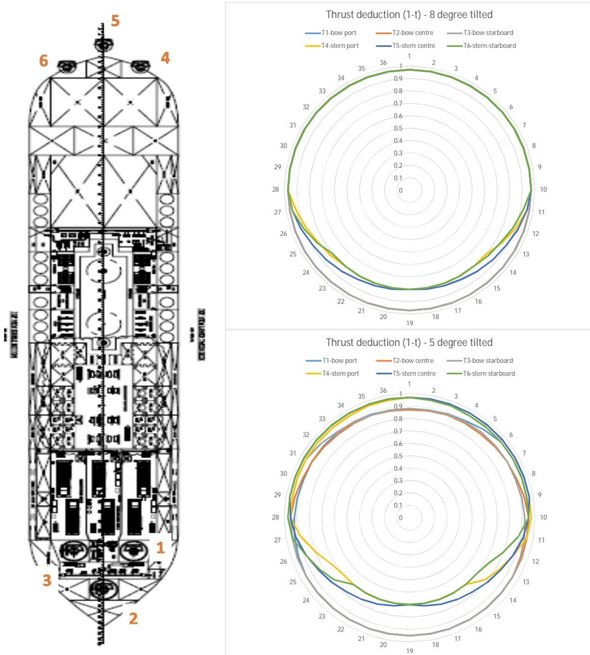
Figure 6: thruster performance including thruster-hull interaction losses
