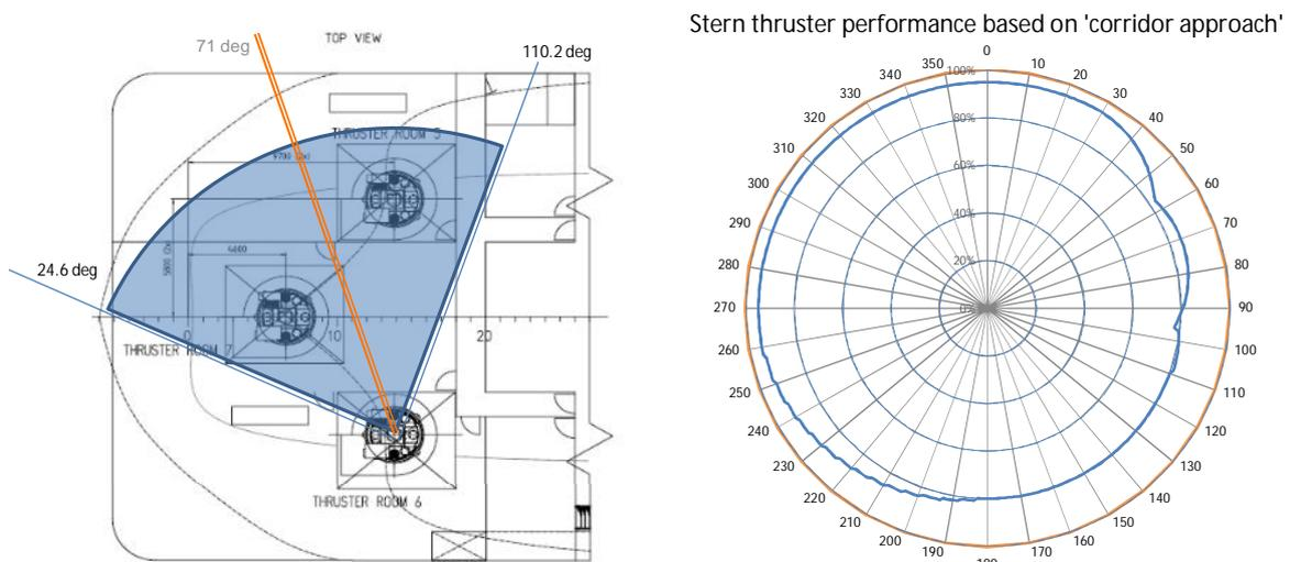
Figure 11: concept of Corridor approach and updated performance of thruster DP-capability
