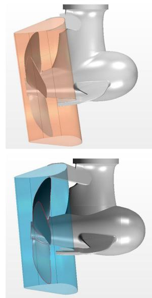
The performance in DP mode, based on the ratio of total thrust/power (T/P) can be evaluated with the so-called Merit Coefficient (MC).
