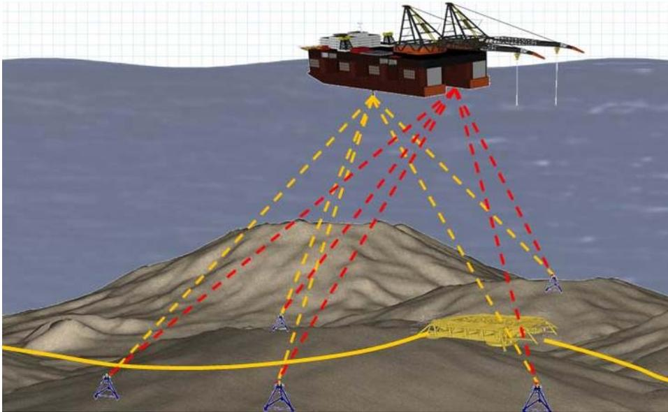
**Figure 5 : A dual independent acoustic system sharing a seabed array with Multi-User transponders**
