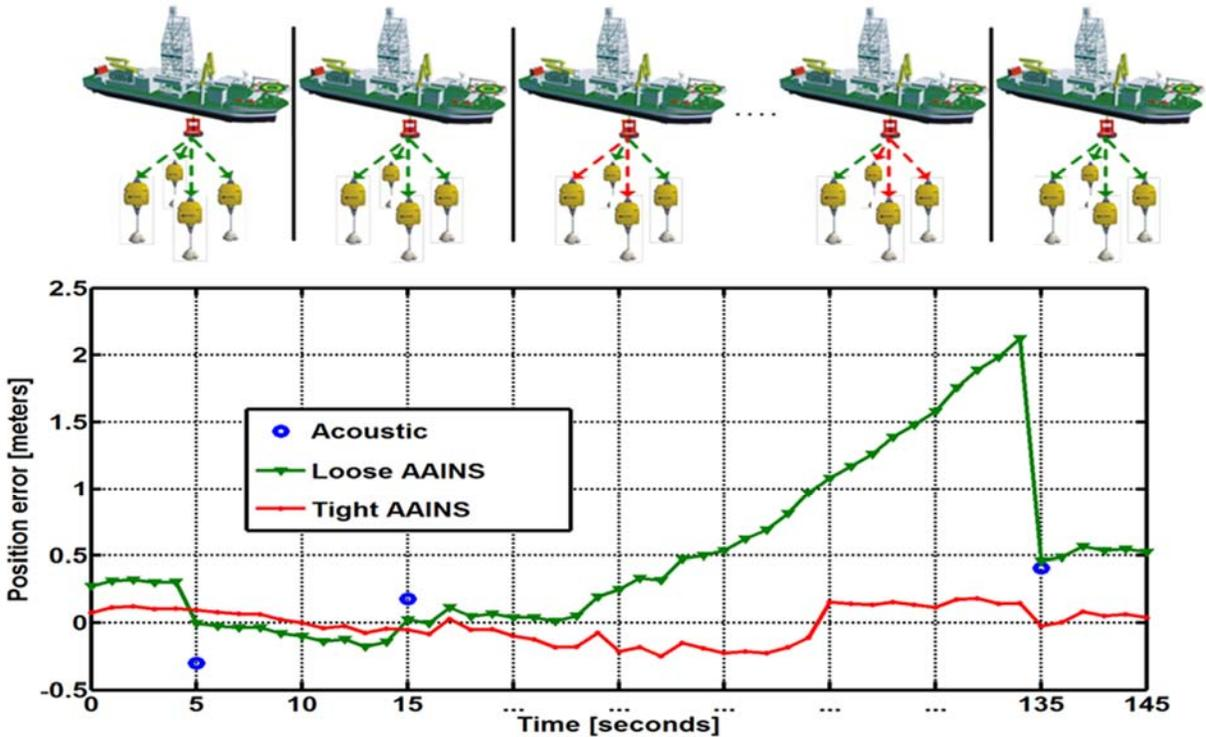
Figure 3 : Fault ride through advantage of tightly coupled
