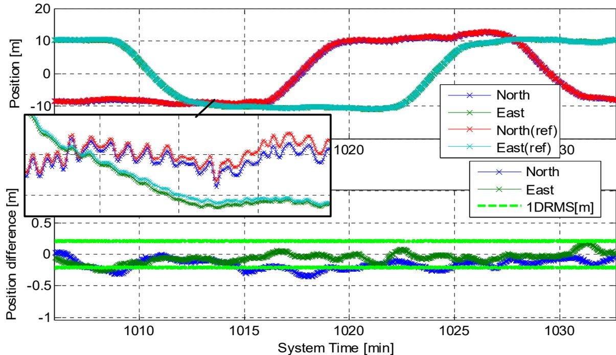
**Figure 4 : Accuracy with a reduced number of transponders**
