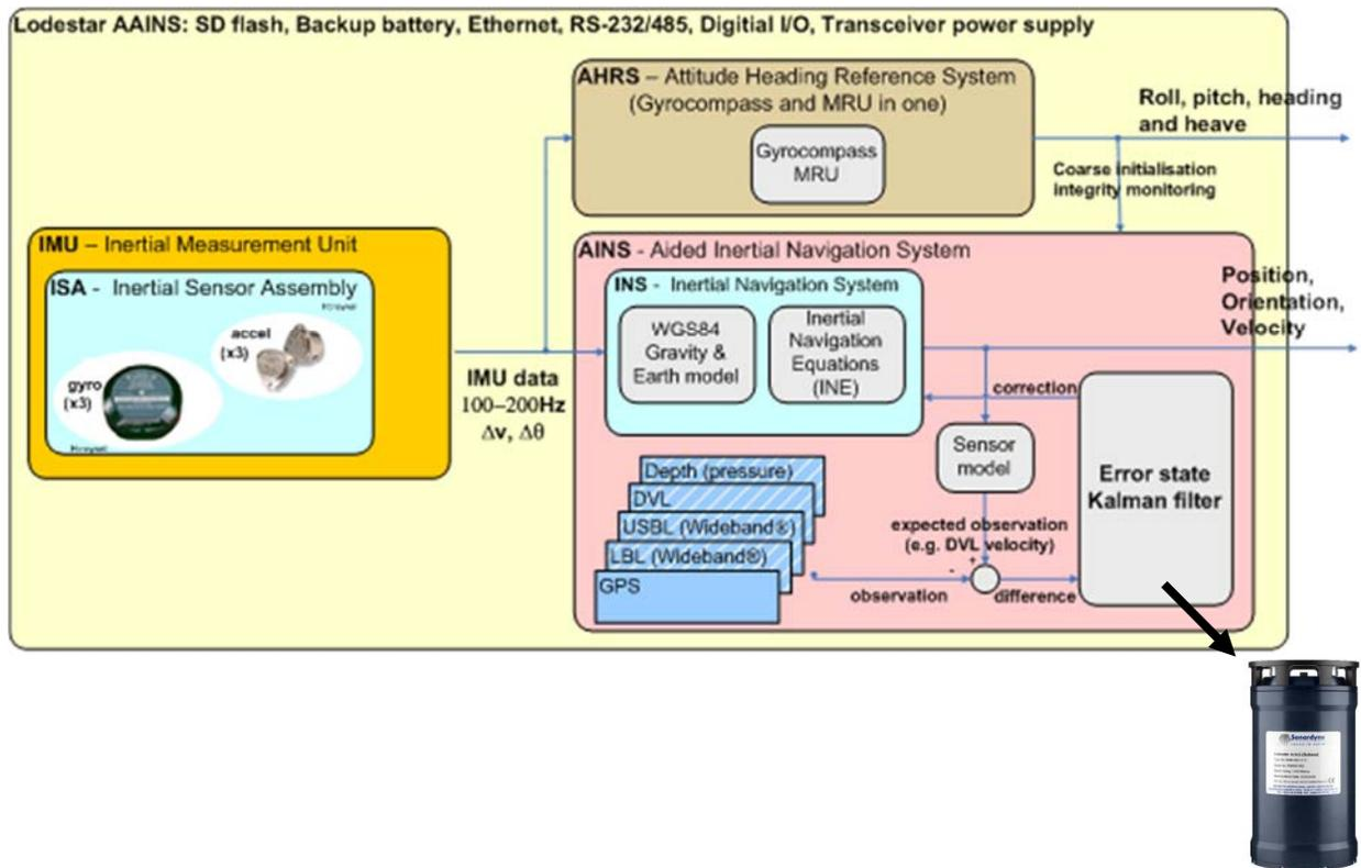
Figure 7: Independent AHRS and INS output
