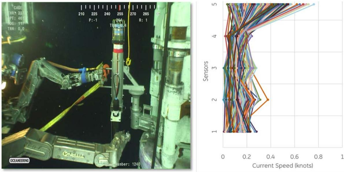
**Figure 8 : Current data collected by SMART transponders**
