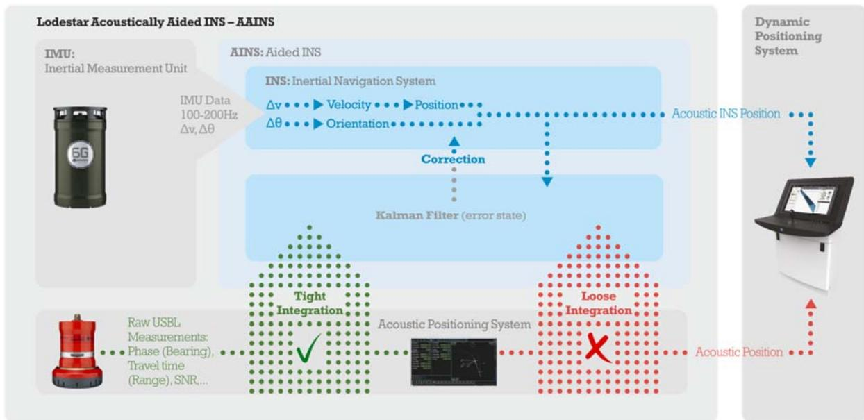
**Figure 2 : Tight and loosely coupled architectures**
