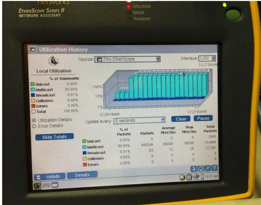
Figure - 3 Multicast Network Storm
