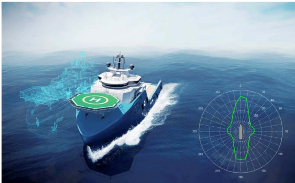
Figure 1: DP vessel and capability plot indicating the vessels station keeping ability
