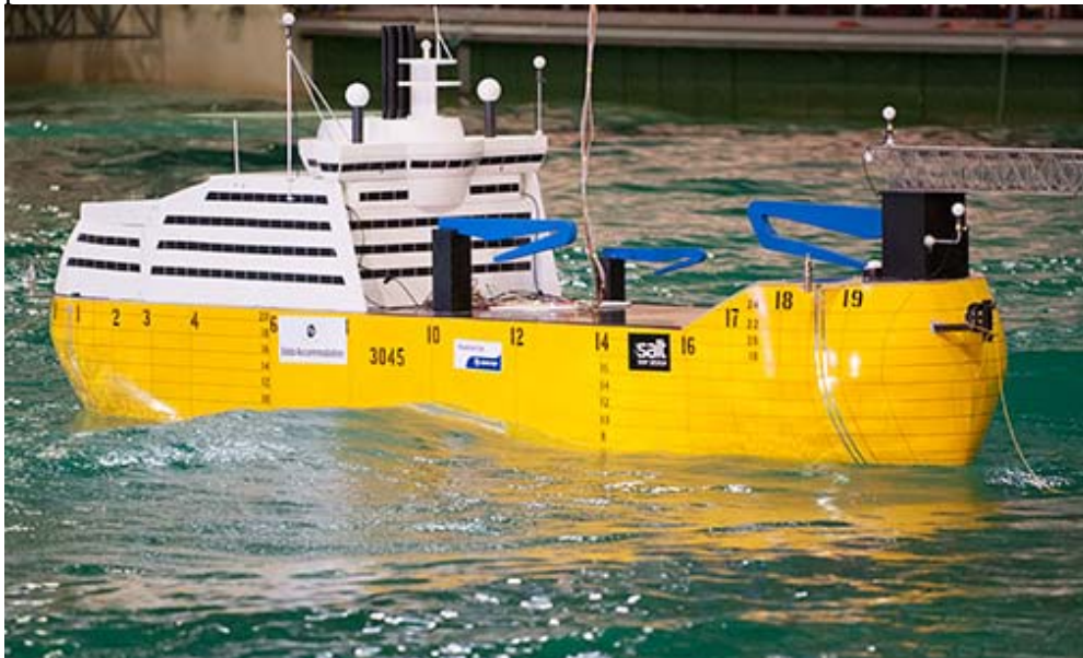
Figure 4, picture of the model vessel from the basin test where the modified control strategy was tested. Courtesy of Marintek.
