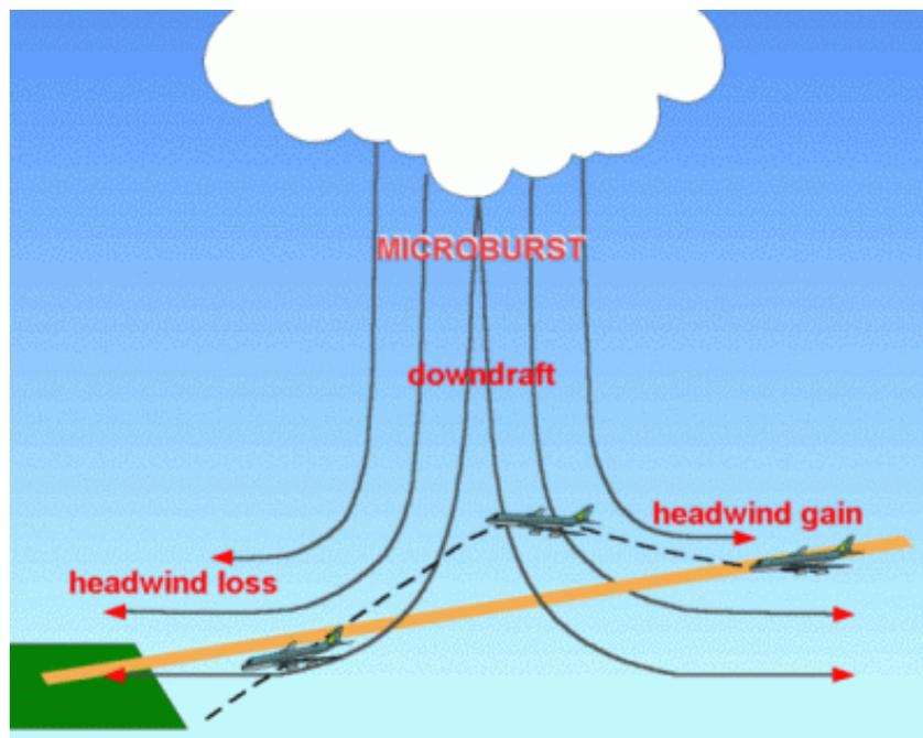
Figure 2: Diagram of microburst and its effects on aircraft
