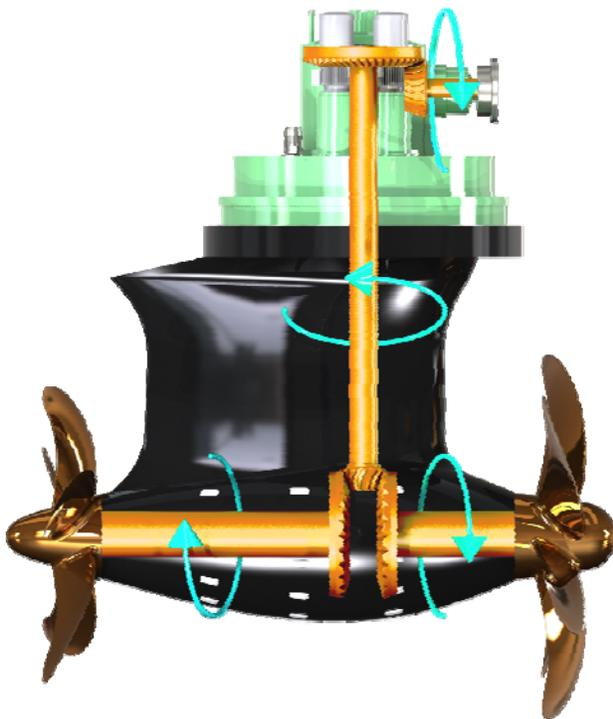
Figure 4 – Mechanical principle of the Dual-End CRP.
