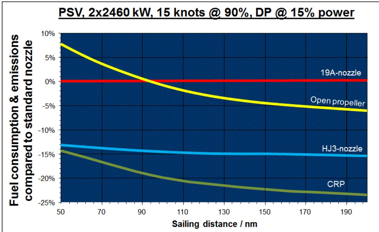
Figure 3 – A case study: Difference in fuel consumption of a DP vessel with different propulsive unit types, relative to a vessel with conventional nozzles.
