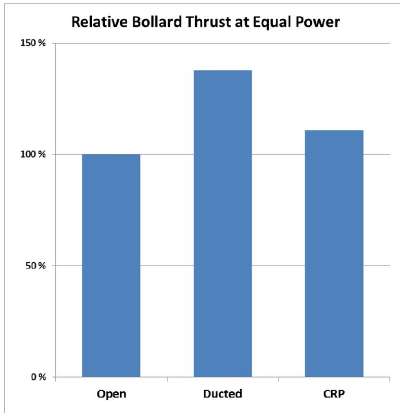
Figure 2 – Approximate relative bollard thrust of propulsive units.
