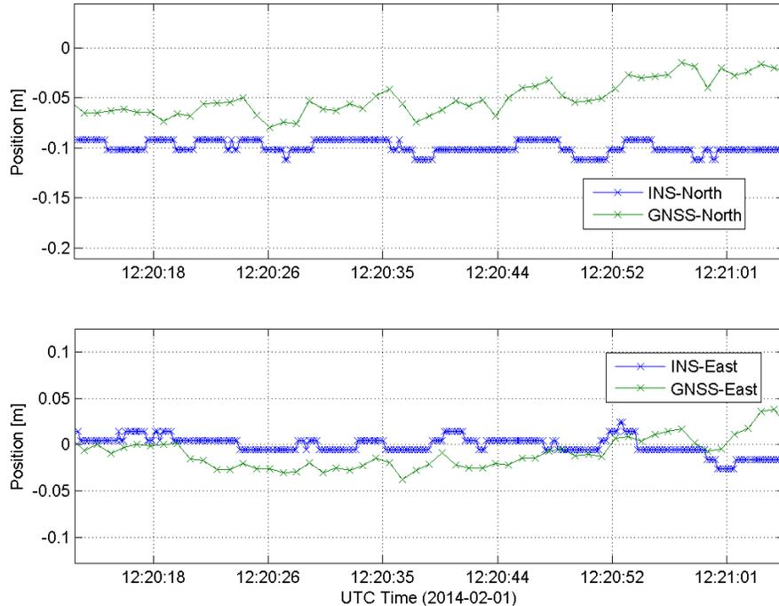
**Figure 3 : Simply adopting legacy interfaces can cause "freeze alarms" in some DP systems due to the different characteristics of INS data**
