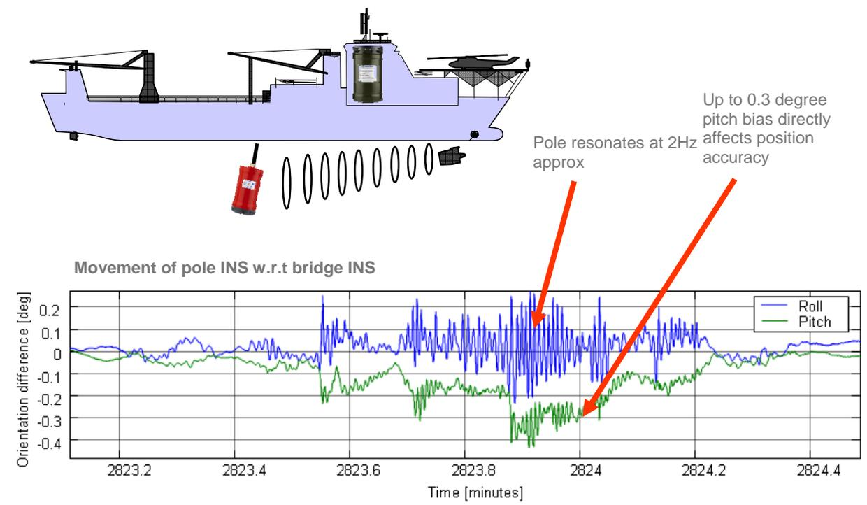
**Figure 9: Movement of pole w.r.t. Bridge INS**
