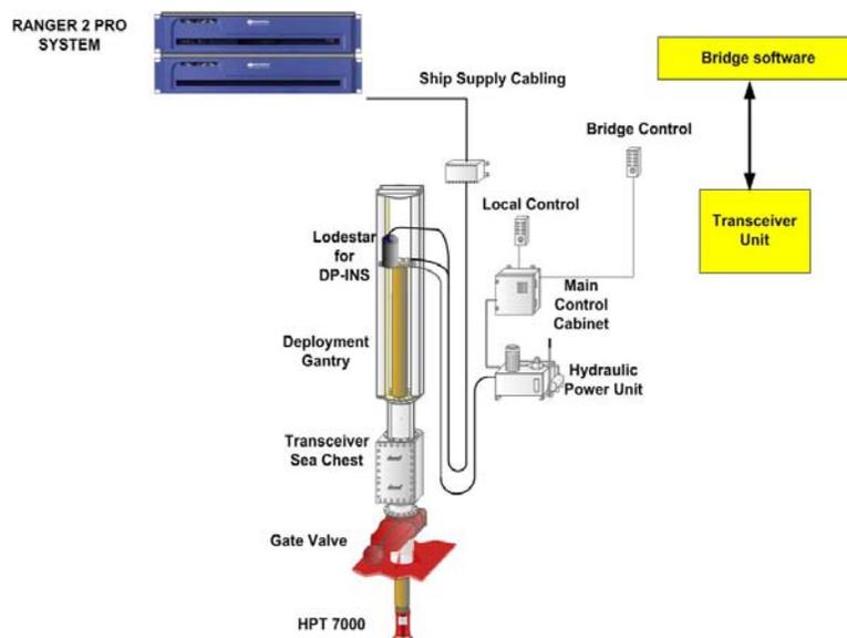
Figure 10 : Complexity of using 3<sup>rd</sup> party deployment poles with proprietary control
