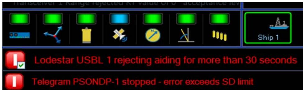
**Figure 5 : Alarms reporting loss of aiding and exceeding error thresholds**
