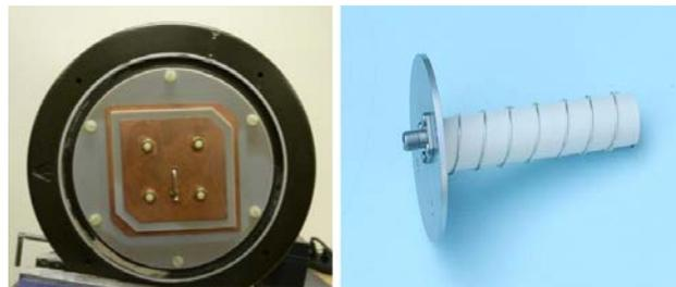
Figure 7 - Antenna Elements (Left - GNSS Patch Element, Right - L-Band Helix Element)
