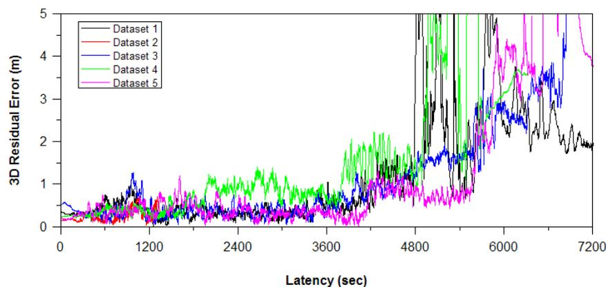
Figure 6 - Effect of Latency on Positioning (High Accuracy PPP)
