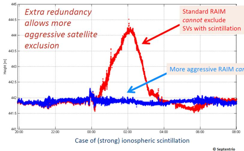
Figure 3 - Improved Position Robustness through Satellite Rejection
