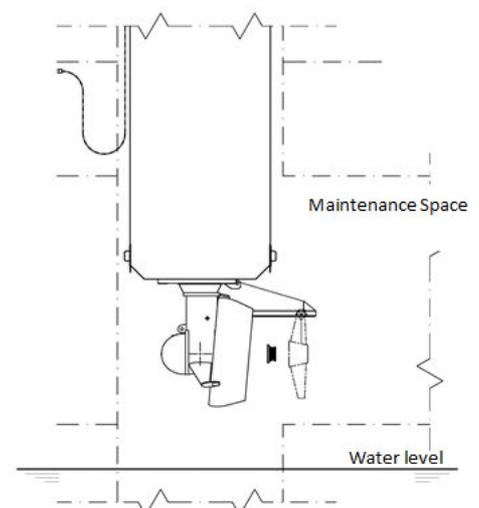
*Fig. Replacement of Propeller Seal*
