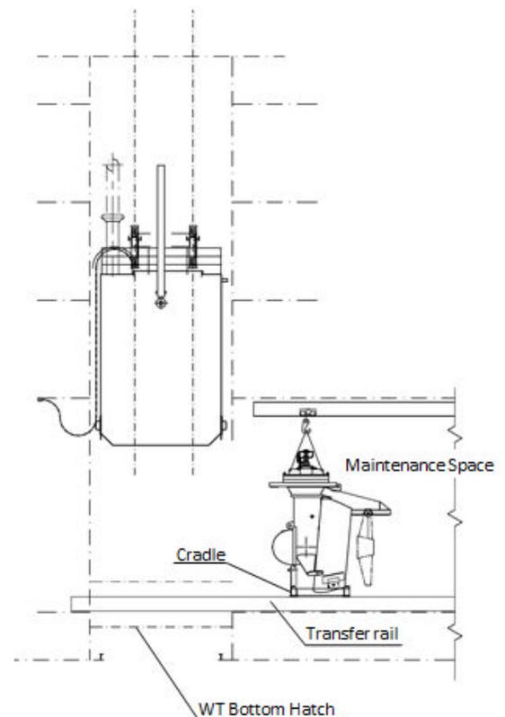
*Fig. Dismantling of Thruster Unit*
