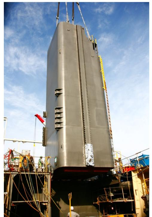
*Fig. Installation preparation of a thruster canister*
