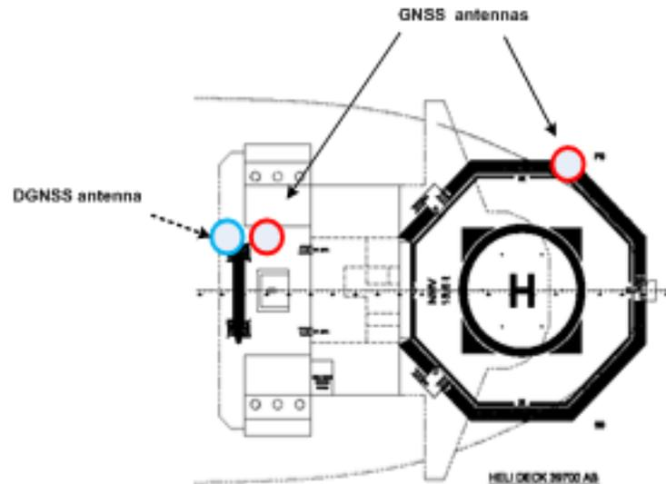
Figure 7: DVC Balder GNSS antenna installation
