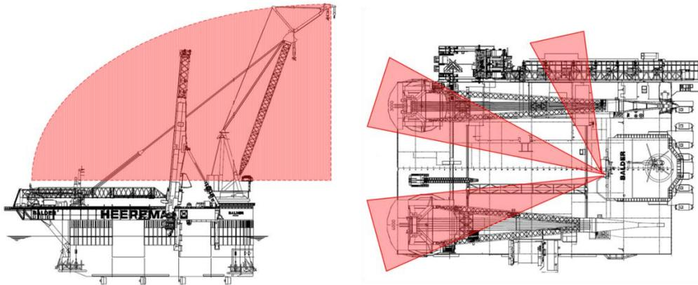
Figure 8: Potential GNSS shadow sectors
