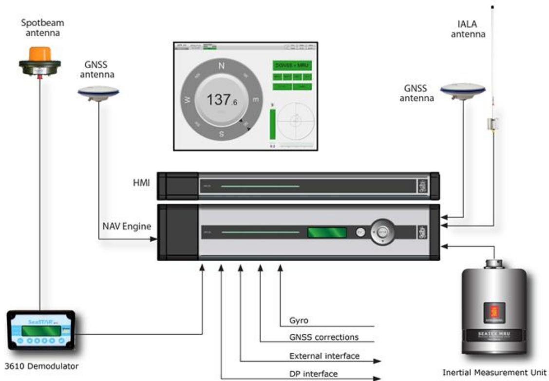
Figure 5: A hybrid GNSS based position, attitude and heading system
