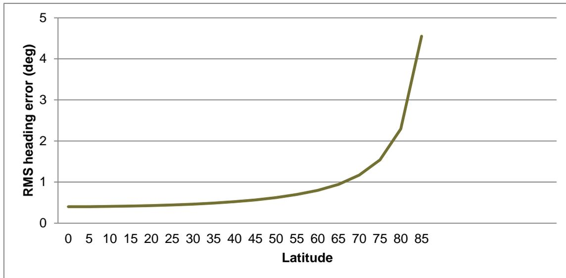
Figure 3: Example of gyro error as function of latitude
