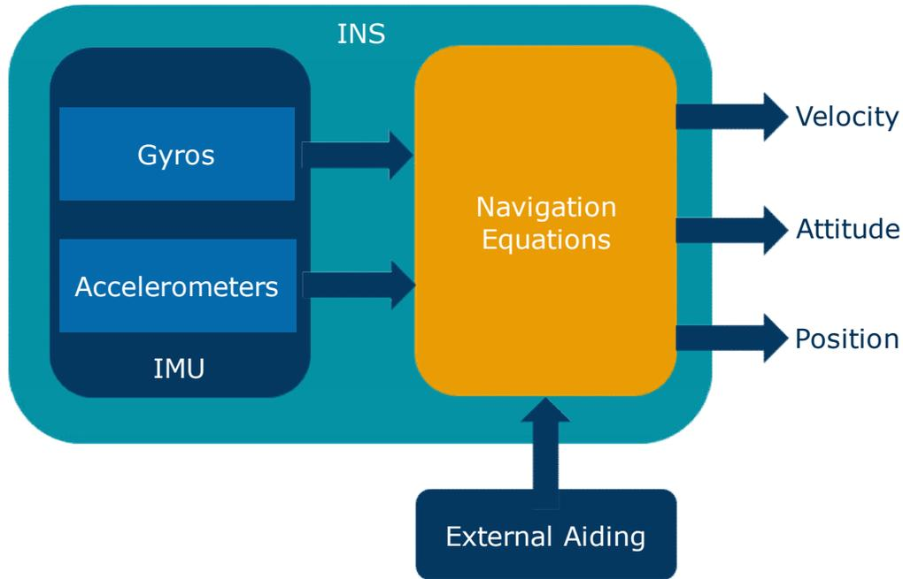
**Figure 6 – Simplified INS Block Diagram**
