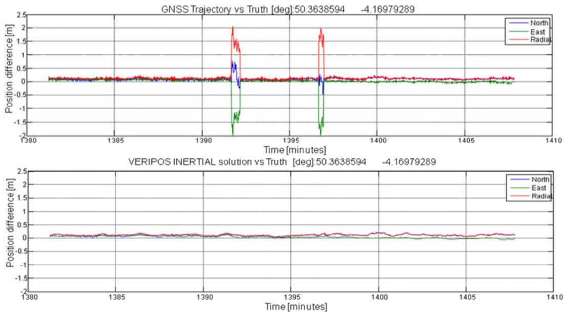
**Figure 13 - Dynamic Vessel Trial Data**
