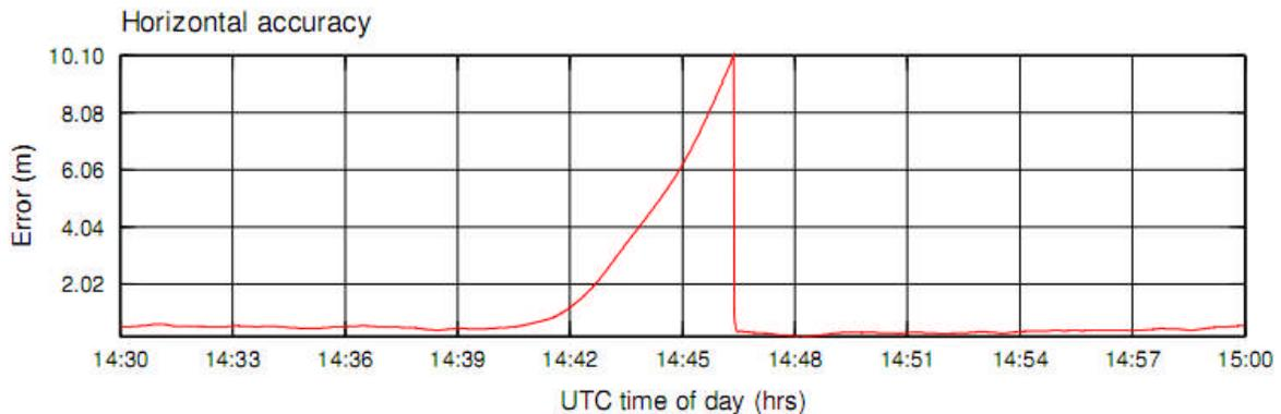
**Figure 11 - Loss of GNSS Measurements**
