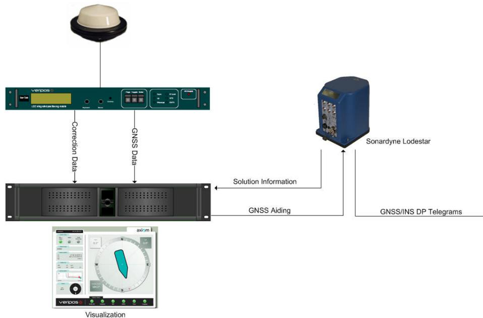
**Figure 9 - Equipment Setup on Vessel**
