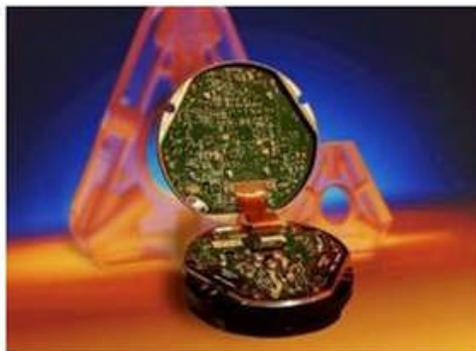
**Figure 5 - Ring Laser Gyro**
