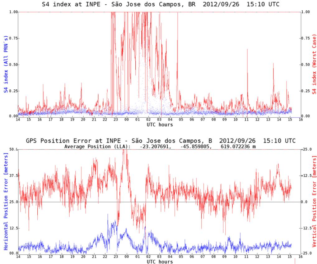
**Figure 3 – L1 GPS Scintillation Monitor in Brazil showing S4 index and Positioning Performance (Cornell University)**
