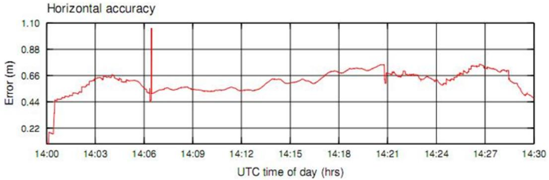
**Figure 12a - GNSS Only Position Solution**
