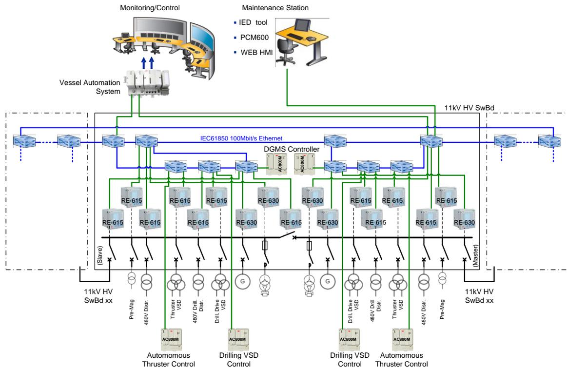
**Figure 3** Typical configuration for a drilling vessel (one of multiple SWBD sections)
