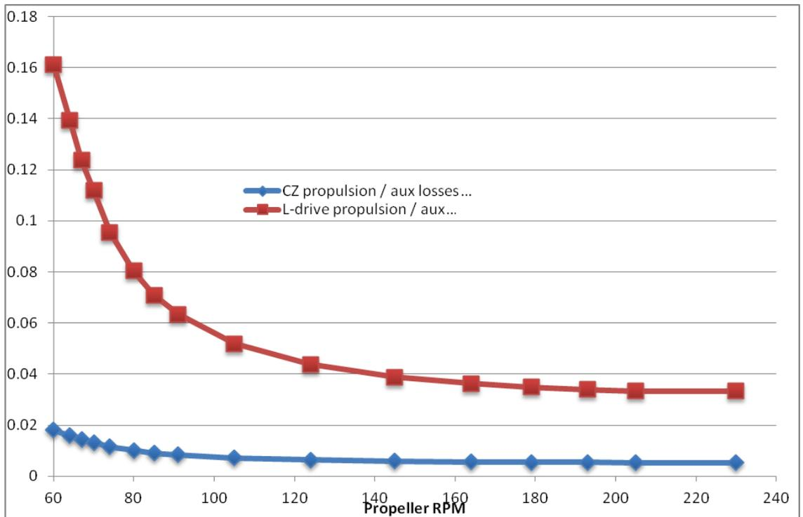
**Figure 11** Auxiliary losses in relation to actual power at specific load point.
