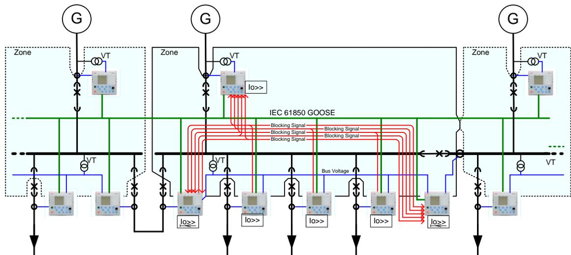
**Figure 5** Example short circuit switchboard zone protection
