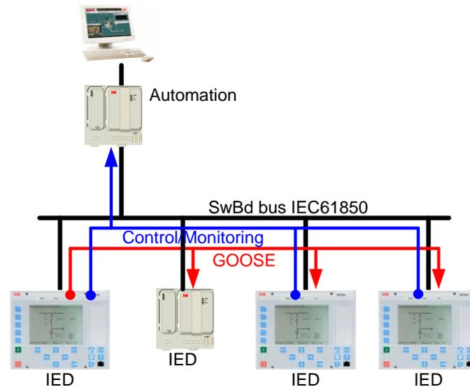
**Figure 2** Typical communication topology [1]
