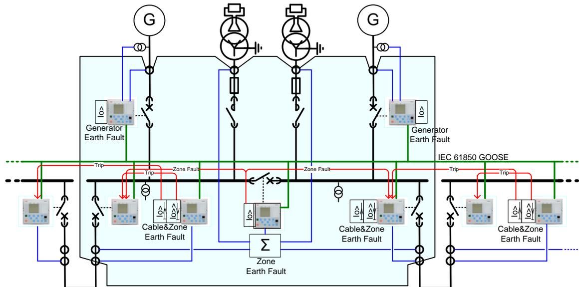
**Figure 4** Example earth fault switchboard zone protection
