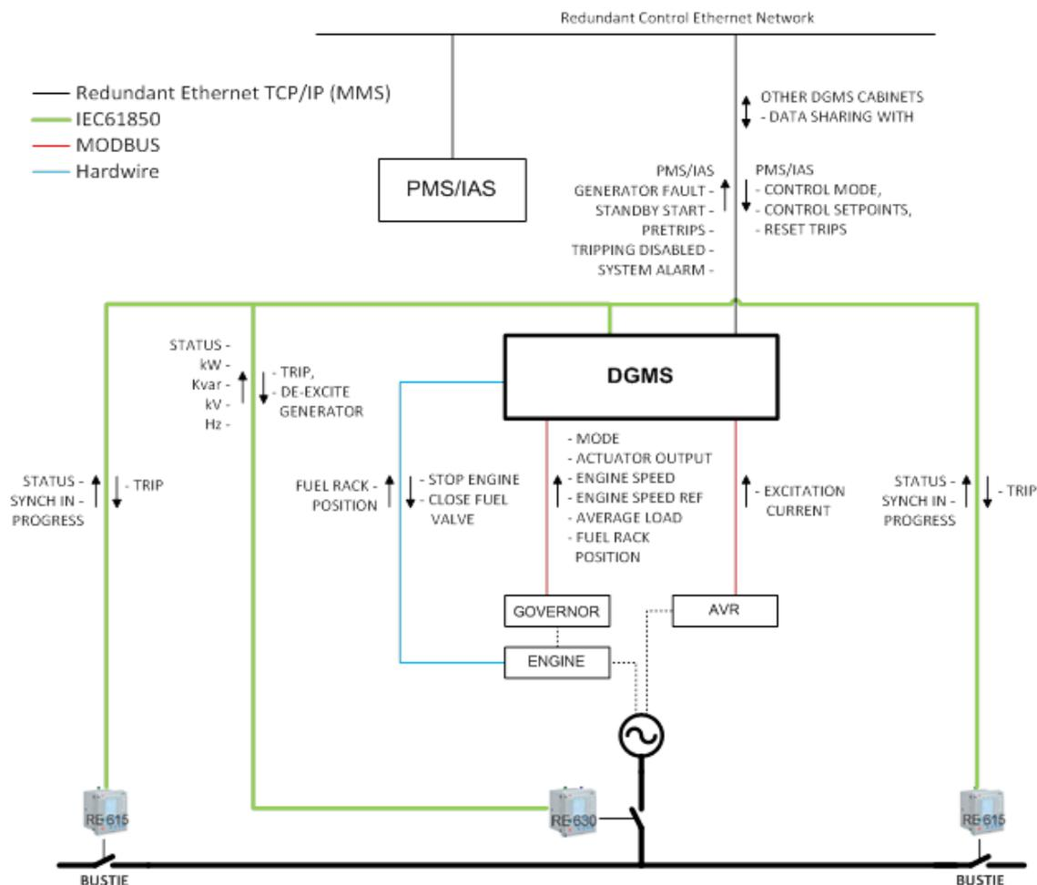
Figure 6 Diesel Generator Monitoring System integration scheme
