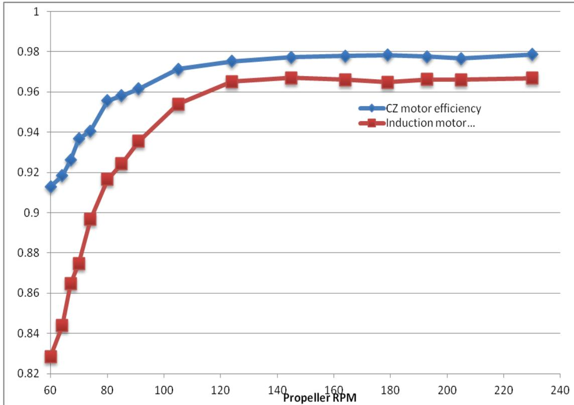
**Figure 10** Electric motor efficiency curves induction motor vs. permanent magnet motor
