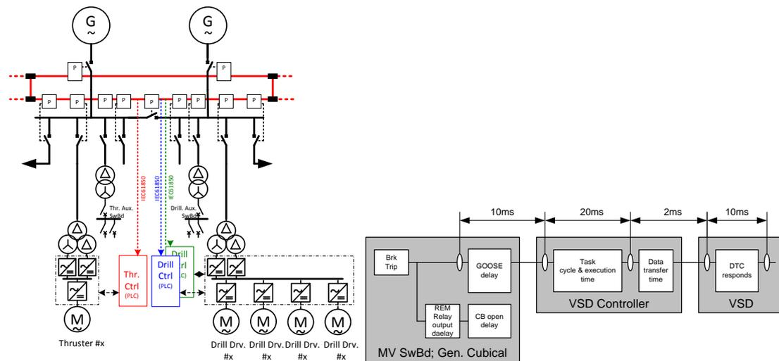
Figure 7 Variable speed drive integration scheme with example time line.
