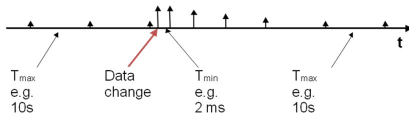
**Figure 1** GOOSE communication time line [1]
