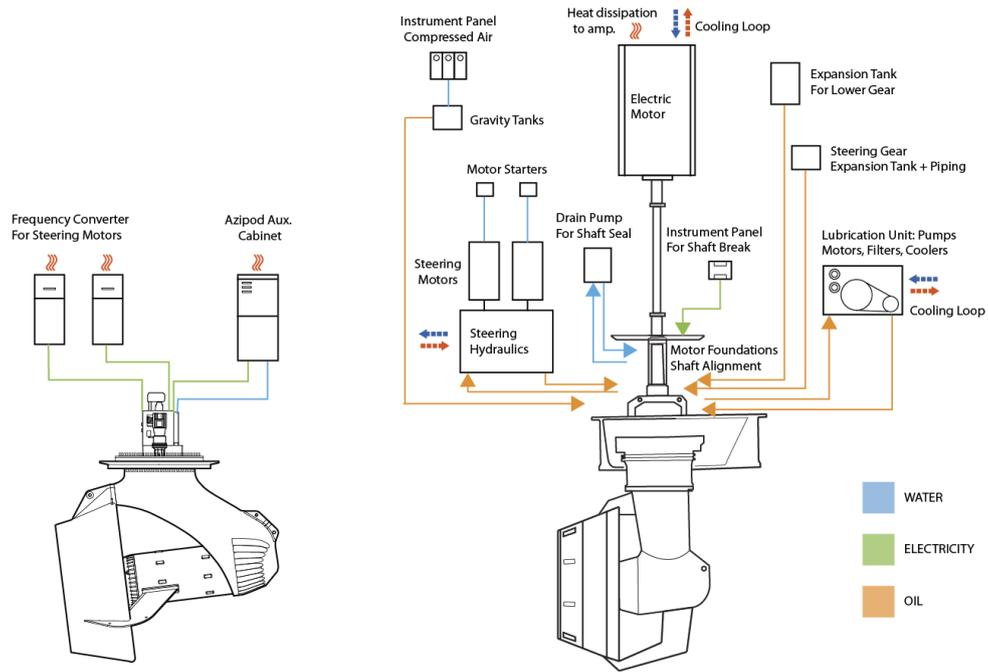
Figure 8 Azipod® CZ vs. Mechanical L-drive with auxiliaries
