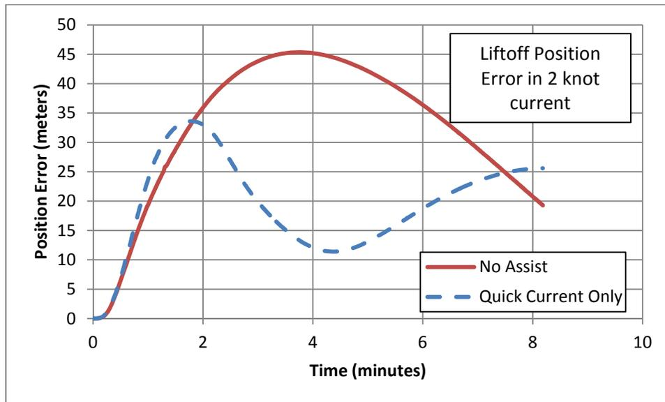
Figure 7. Large Position Losses Possible Without Current Compensation
