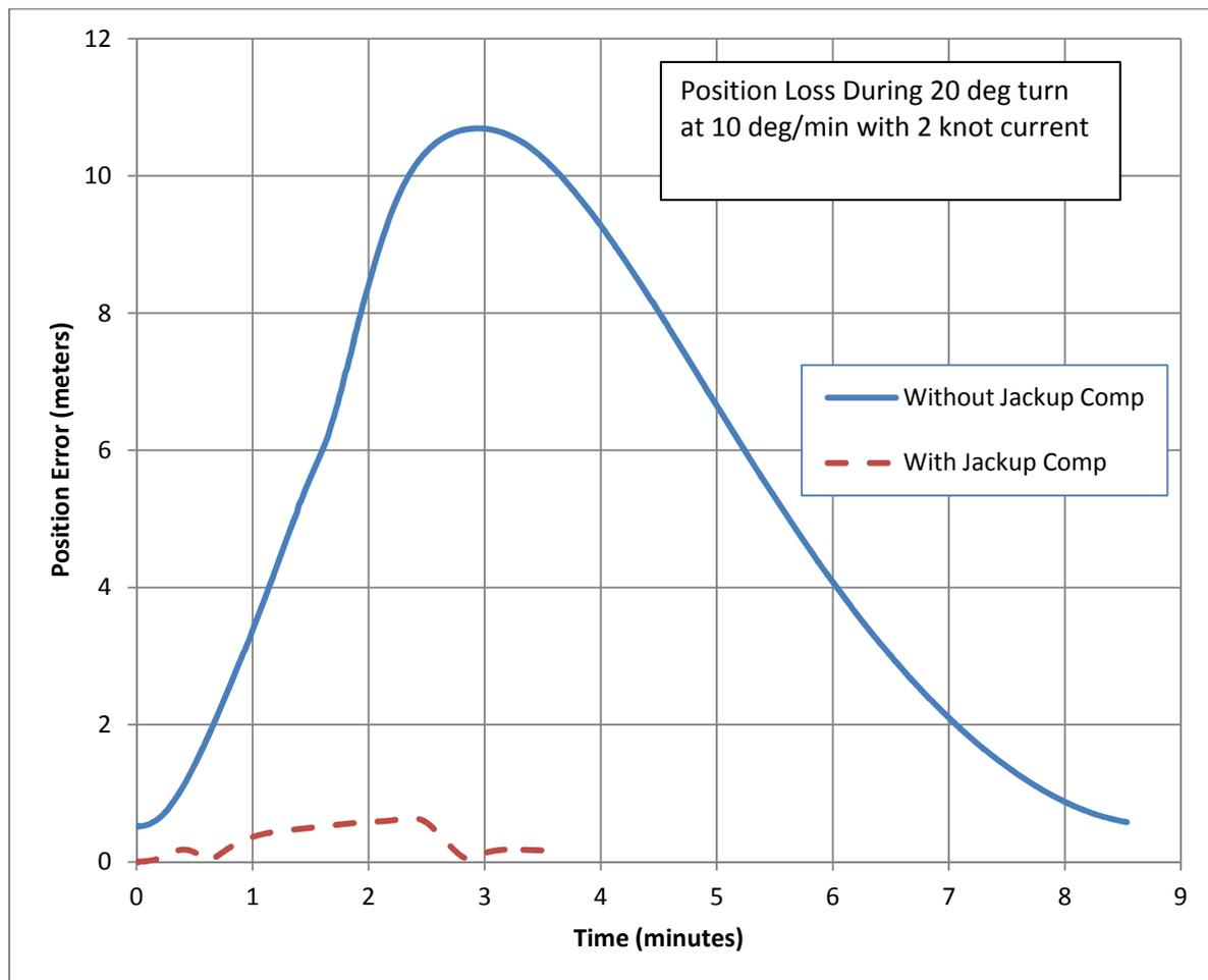
Figure 5. Jackup Compensation Reduces Position Loss During Turn
