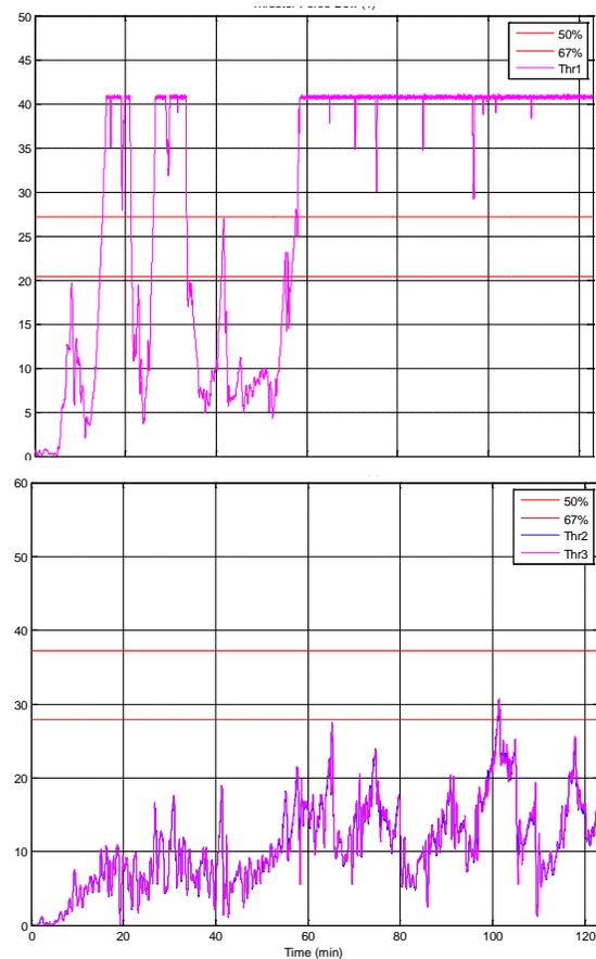
Figure 11: Thruster forces of PRV (ton force) bow (top) and stern (bottom) for the full test series
