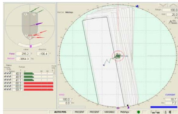
Figure 8: ADS operating at 10° ice drift angle
