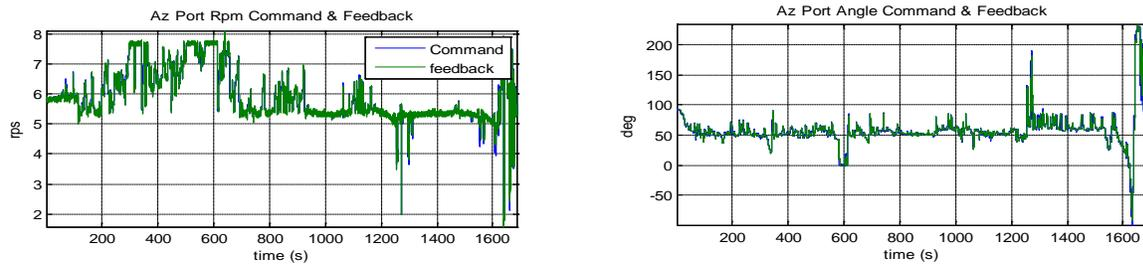
Figure 16: Port stern thruster speed (rps) and azimuth (deg)
