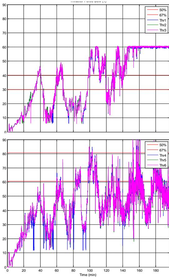
Figure 10: Thruster forces of ADS (ton force) bow (top) and stern (bottom) for the full test series
