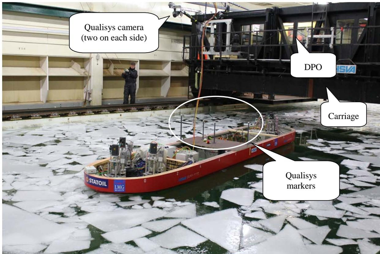
Figure 1: Test setup
