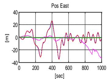
Figure 12: Transverse position using simulated "Open water DP" (red) compared to recorded data (magenta)
