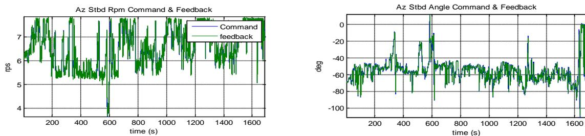
Figure 17: Starboard stern thruster speed (rps) and azimuth (deg)
