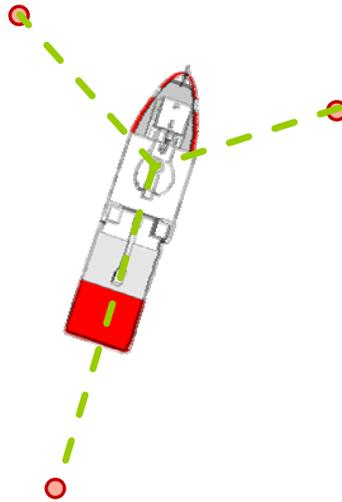
Figure 3 – Position Aiding (minimum 3 ranges)
