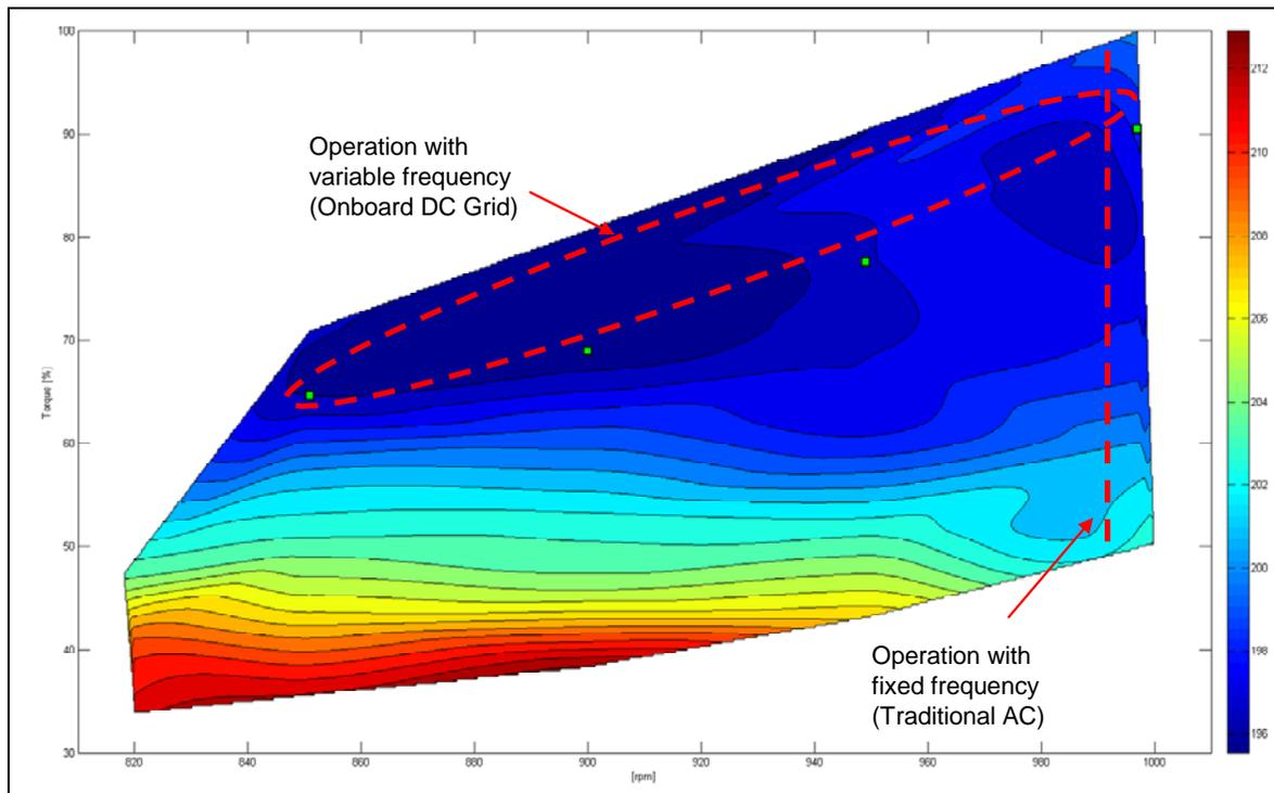
**Fig. 3: SFOC as function of RPM and torque.**
