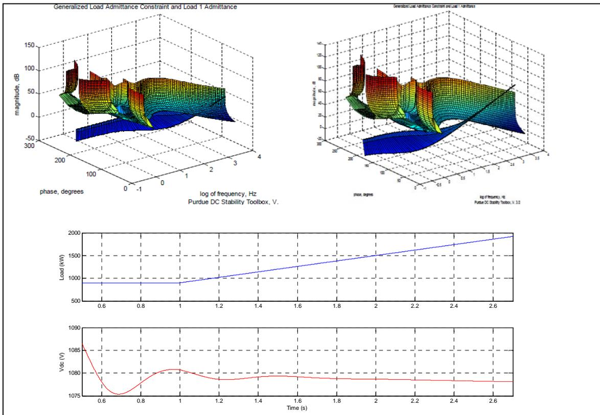
**Fig. 4: Stability plot and simulation of Onboard DC Grid.**
