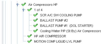
**Figure 5 Illustration of which power consumers that need to be powered in order to operate the HP Air Compressors**
