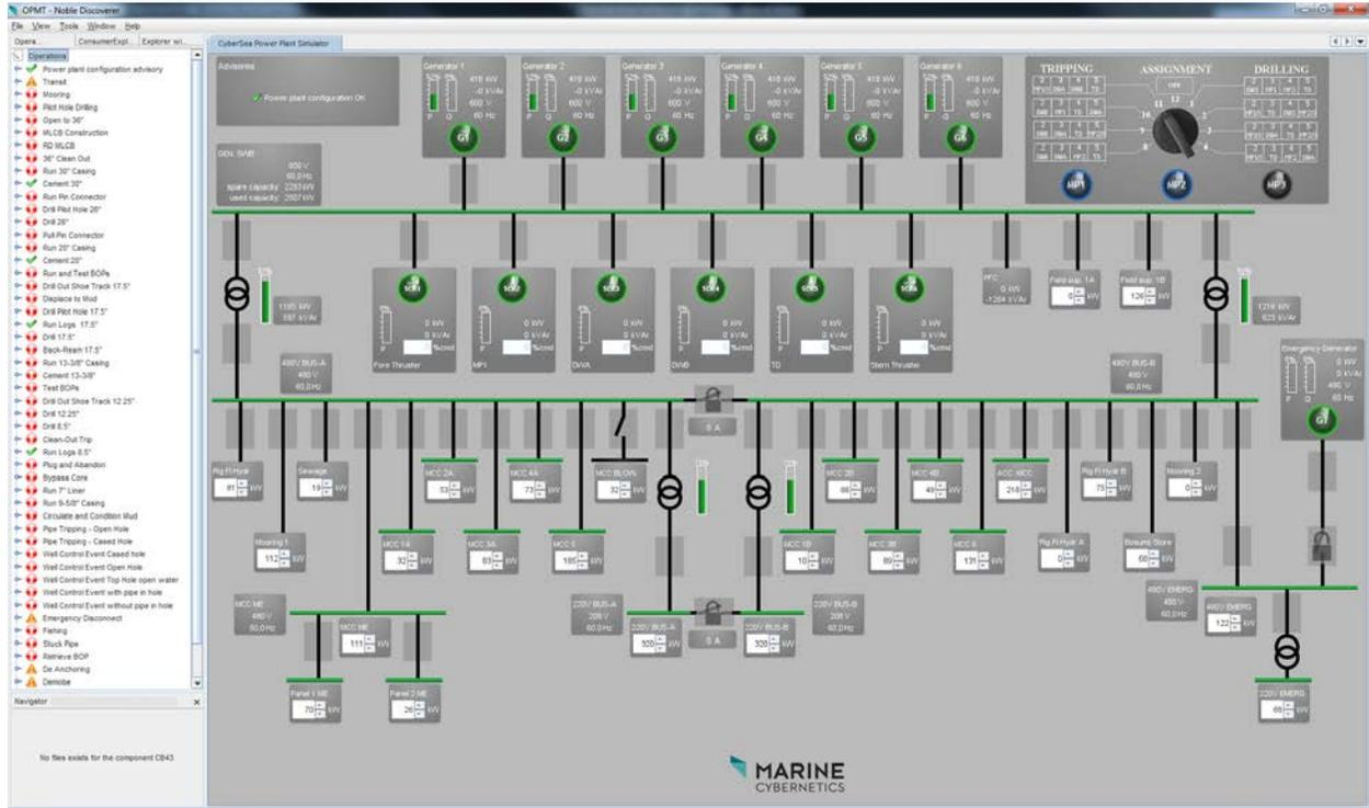
**Figure 3 User interface.** This page shows the power plant configuration page. The configuration of the DP system (e.g. pos.ref. and sensors) will be shown in a separate page.
