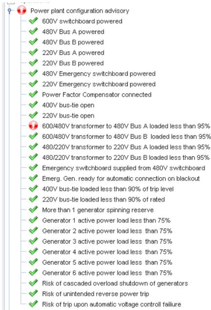
**Figure 9 Example of implemented power plant advisory. The red icon indicates that an advisory condition is not fulfilled with the configuration being simulated.**
