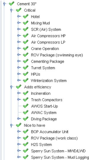
**Figure 4 Illustration of operation dependencies for cementing 30” casing**
