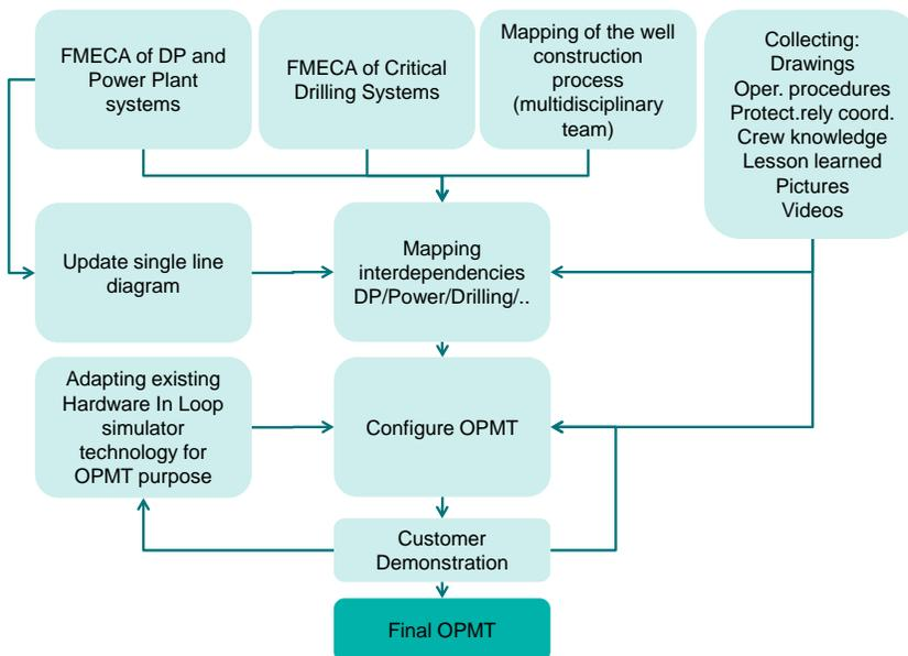
**Figure 1** Illustration of work process and methodology for making an OPMT for an existing vessel (the pilot project).
