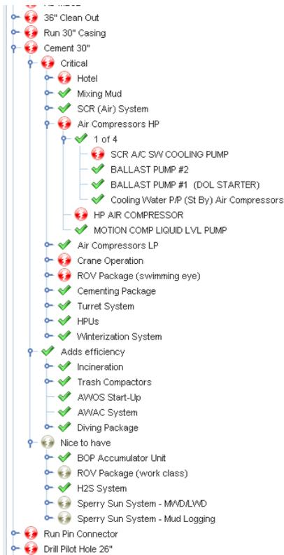
**Figure 7 Consequences of losing MCC2A.** The red icons indicate that critical equipment has lost, gray icons indicate loss of nice-to-have equipment.
