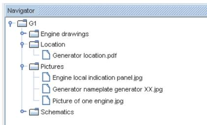
**Figure 10 Example list showing information available on generator G1. The information is accessed by clicking on the generator symbol in the single line diagram.**
