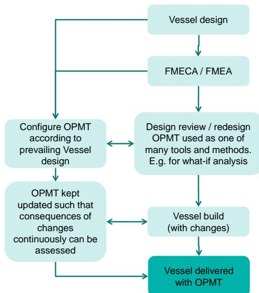
**Figure 2** Illustration of how the work process and methodology for making an OPMT for a new vessel could look like.
