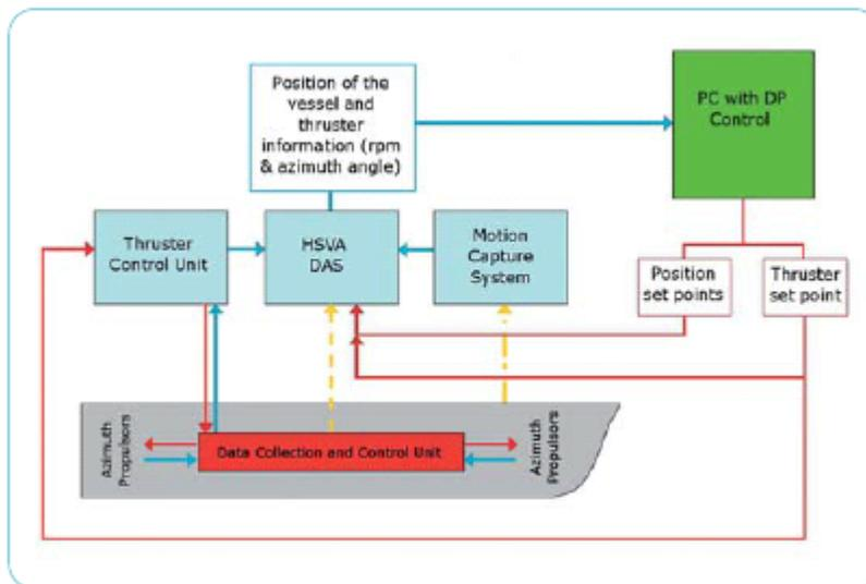
Figure 3: Interface between tank instrumentation and DP system
