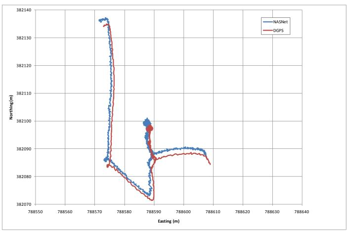
Effects of SV error and weak geometry on positioning accuracy Stability, latency and update rate unaffected
