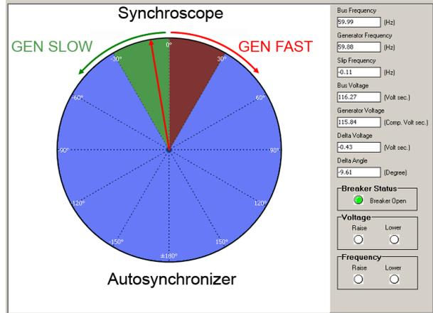
Fig. 8 Automatic Synchronization
