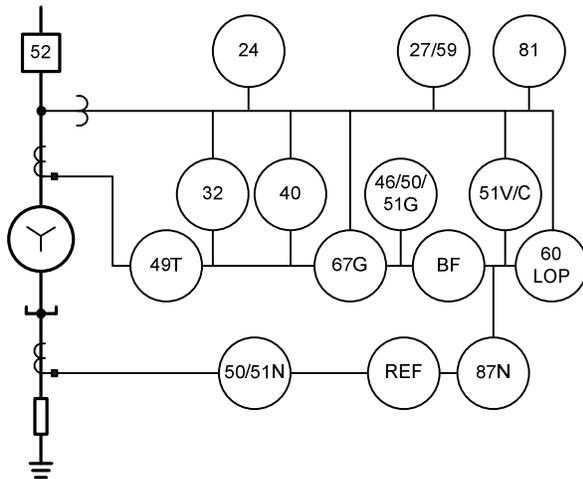
Fig. 7 Standard Features of Generator Protection Relay
