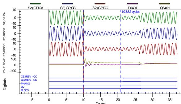
Fig. 11 Example Fault Analysis for the Three-Phase Fault
