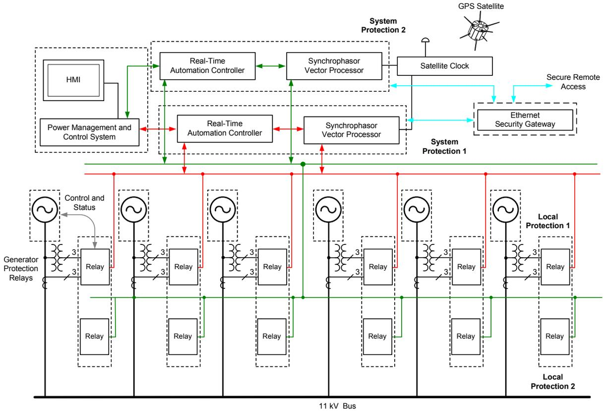
Fig. 5 Proposed Solution—Redundant Protection
