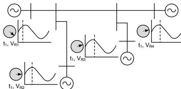
Fig. 12 Synchrophasor Measurement
