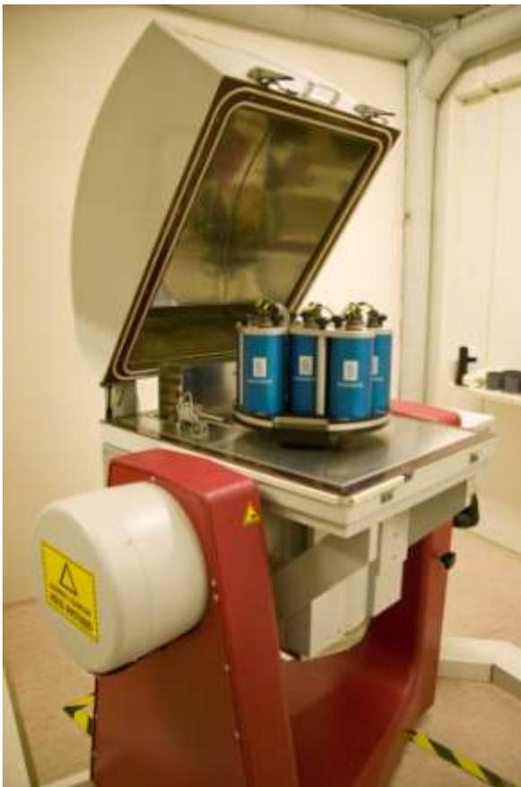
**Figure 9: Position/Rate table for IMU testing**
