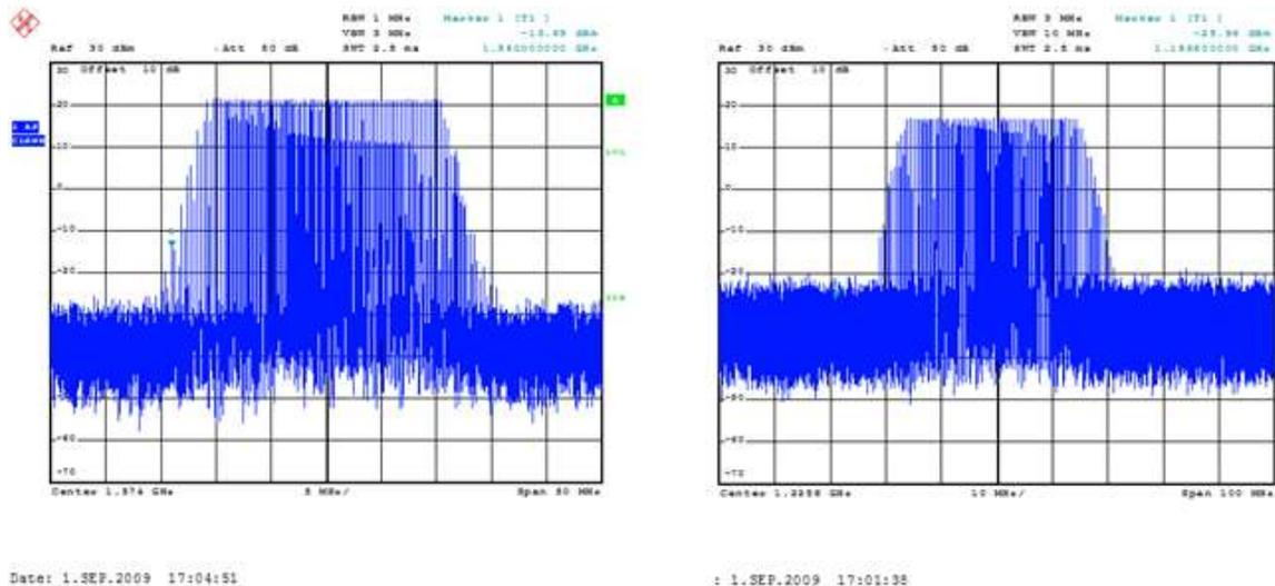
**Figure 4: GPS jammer L1 and L2 signal**
