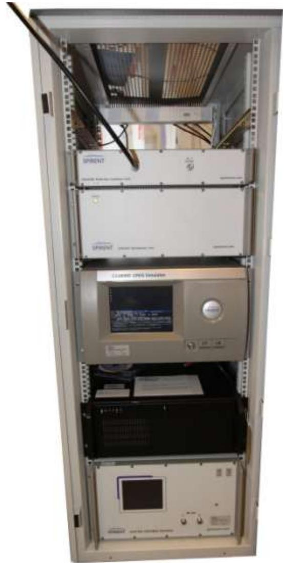
**Figure 8: GPS & Glonass simulator equipment**
