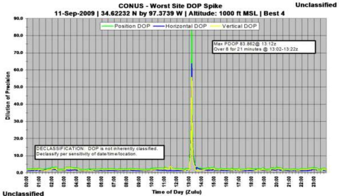
Figure 2: USCG Navigation Center high HDOP warning
