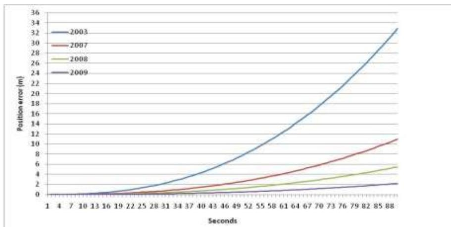
**Figure 12: Position error caused by angular random walk**
