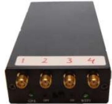
**Figure 3: GPS jammer**
