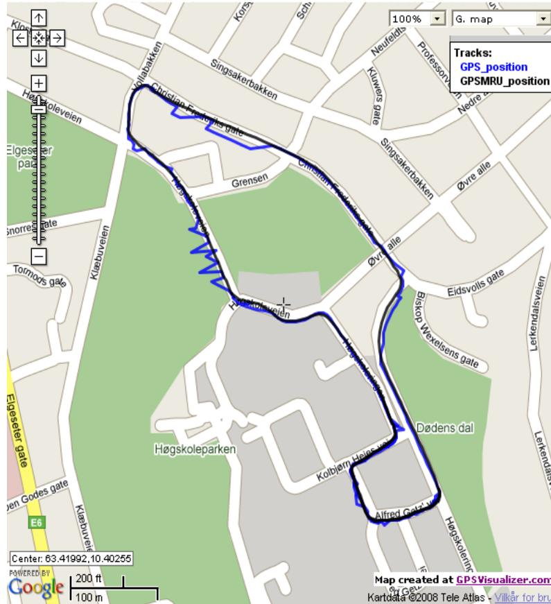
Figure 6: GNSS and IMU/GNSS position driving under dense foliage
