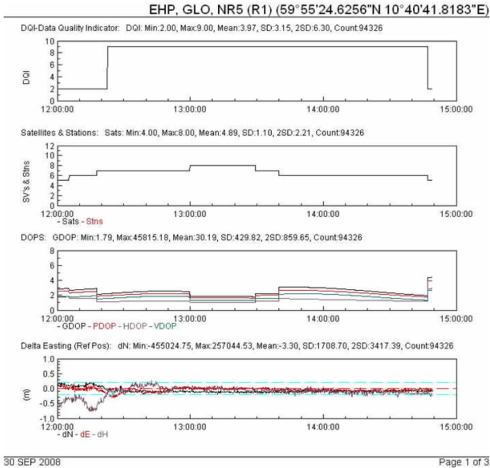
Figure 5: GLONASS only orbit/clock solution in Oslo 30 Sept2008.
