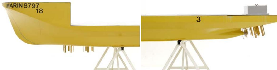
*Figure 3: Photographs with fore and aft ship of Mighty Servant equipped with Voith Schneider propellers*
