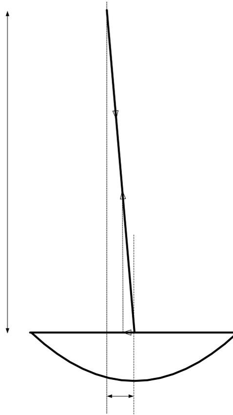
**Figure 3 – Horizontal force due to cable tension**
