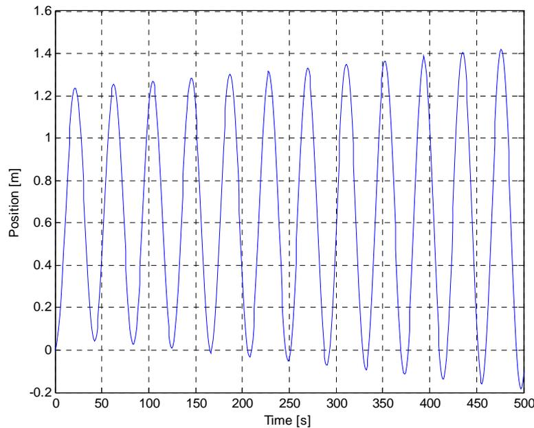
**Figure 4 – Simulated position under normal DP control**
