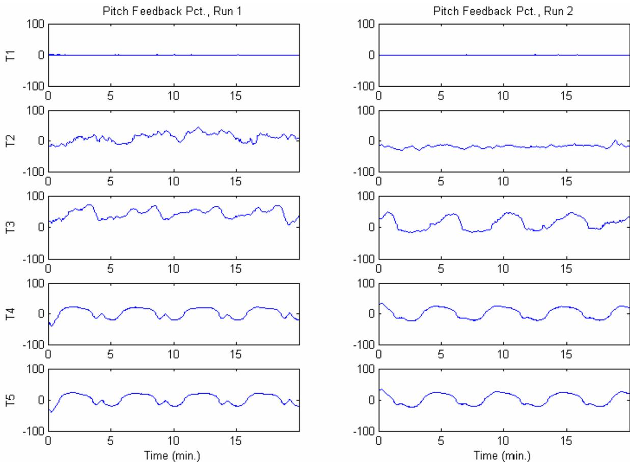
**Fig. 3.** Decoupled surge tests on the full scale vessel: pitch feedback for each of the five propellers, labeled T1-T5.
