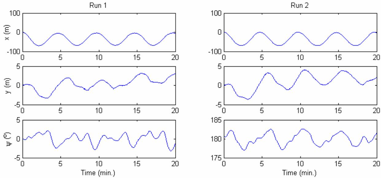
**Fig. 2.** Decoupled surge tests on the full scale vessel: position and heading ( $\psi$ ) data.
