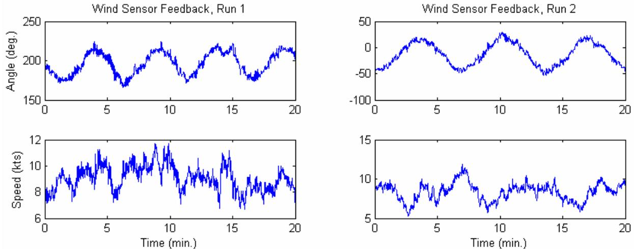
**Fig. 6.** Coupled surge/sway tests on the full scale vessel: wind sensor feedback (relative to the body frame).
