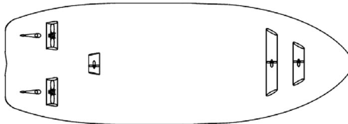
**Fig. 1.** Thruster configuration a typical DP Class 2 supply vessel.
