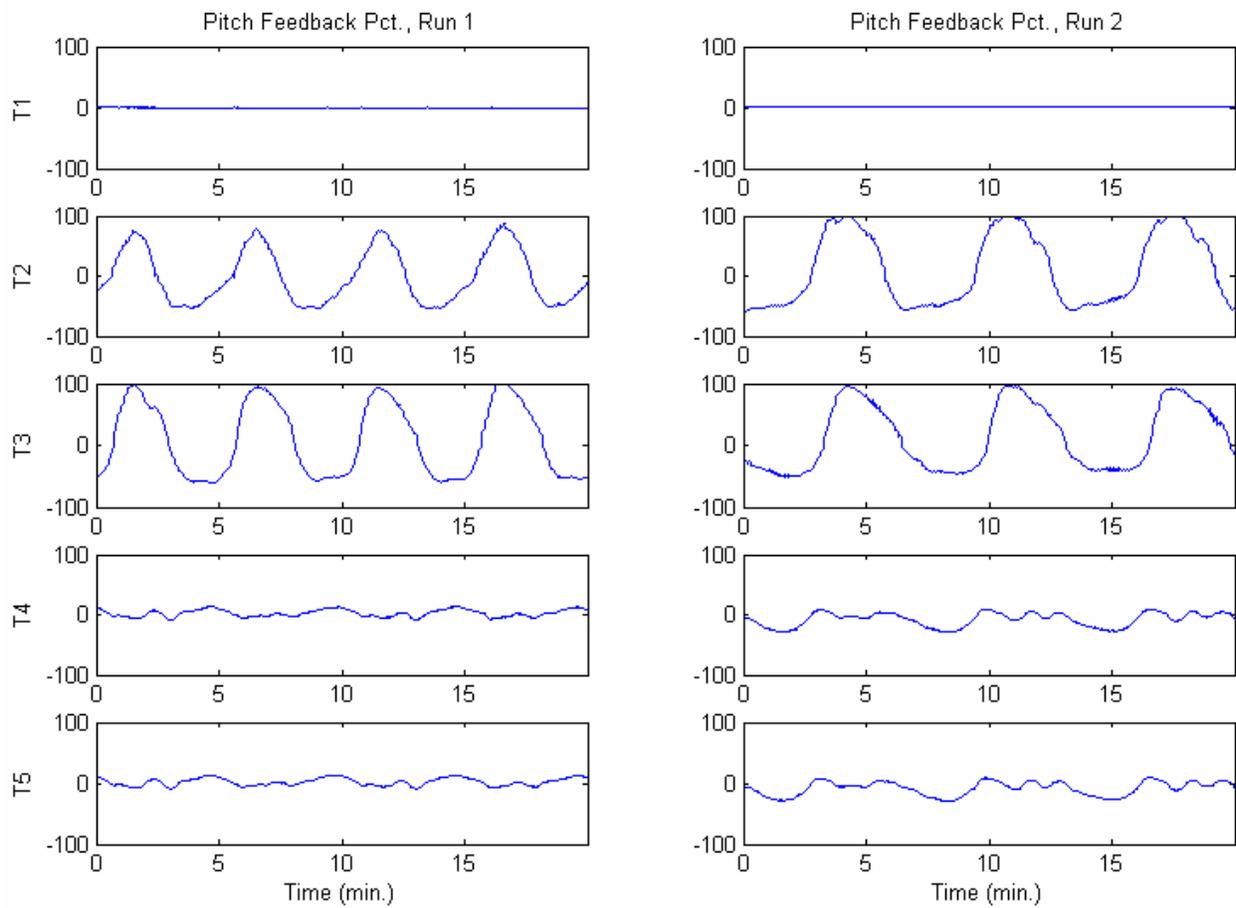
**Fig. 5.** Coupled surge/sway tests on the full scale vessel: pitch feedback for each of the five propellers, labeled T1-T5.
