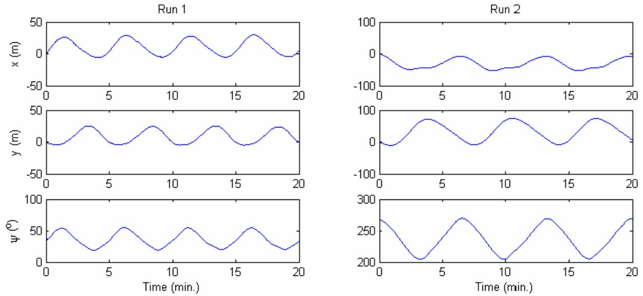
**Fig. 4.** Coupled surge/sway tests on the full scale vessel: position and heading ( $\psi$ ) data.
