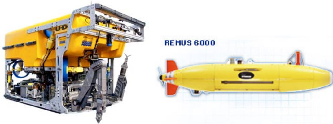
FIGURE 1: Typical ROV and AUV.
