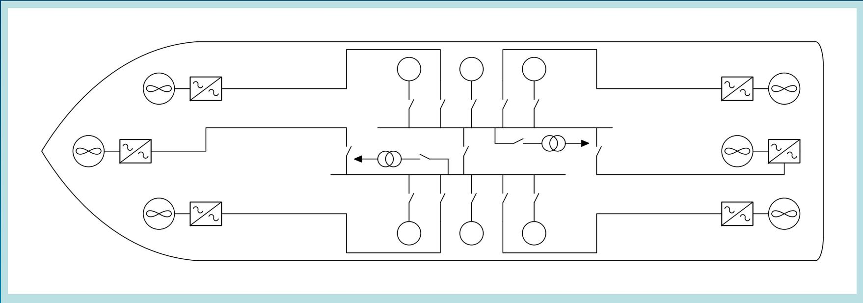
Worst Case Failure - Loss of three generators and three thrusters – **Only one bow thruster available**
