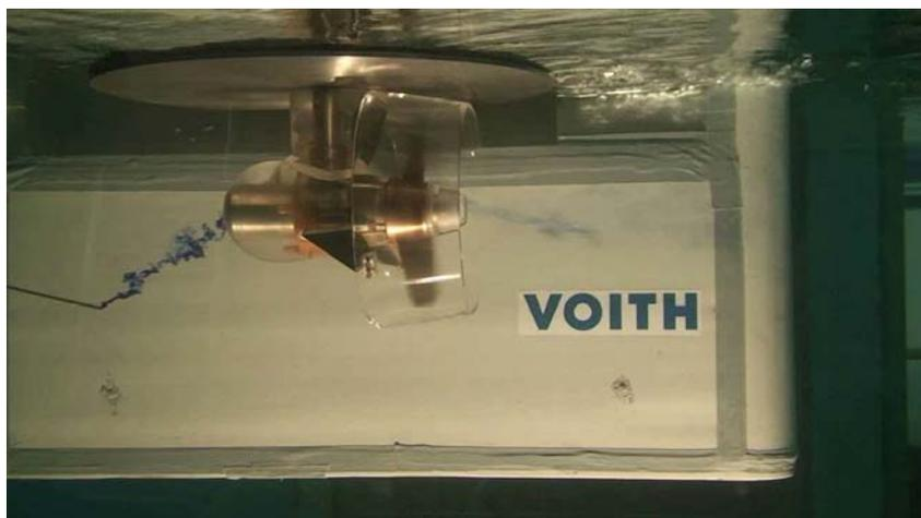
**Fig. 16. Visualization of the flow pattern with ink**
