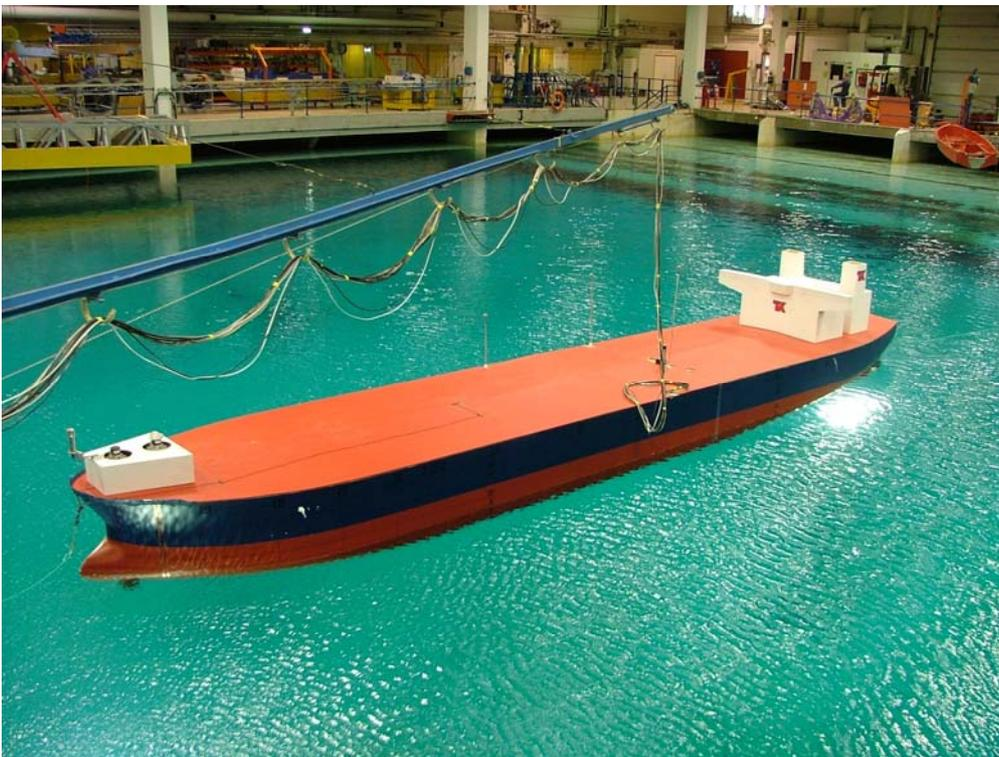
**Figure 10** The 10 meter long model ready for DP testing in Marintek’s Ocean Basin. The model is controlled by an “off the shelf” Kongsberg DP system.
