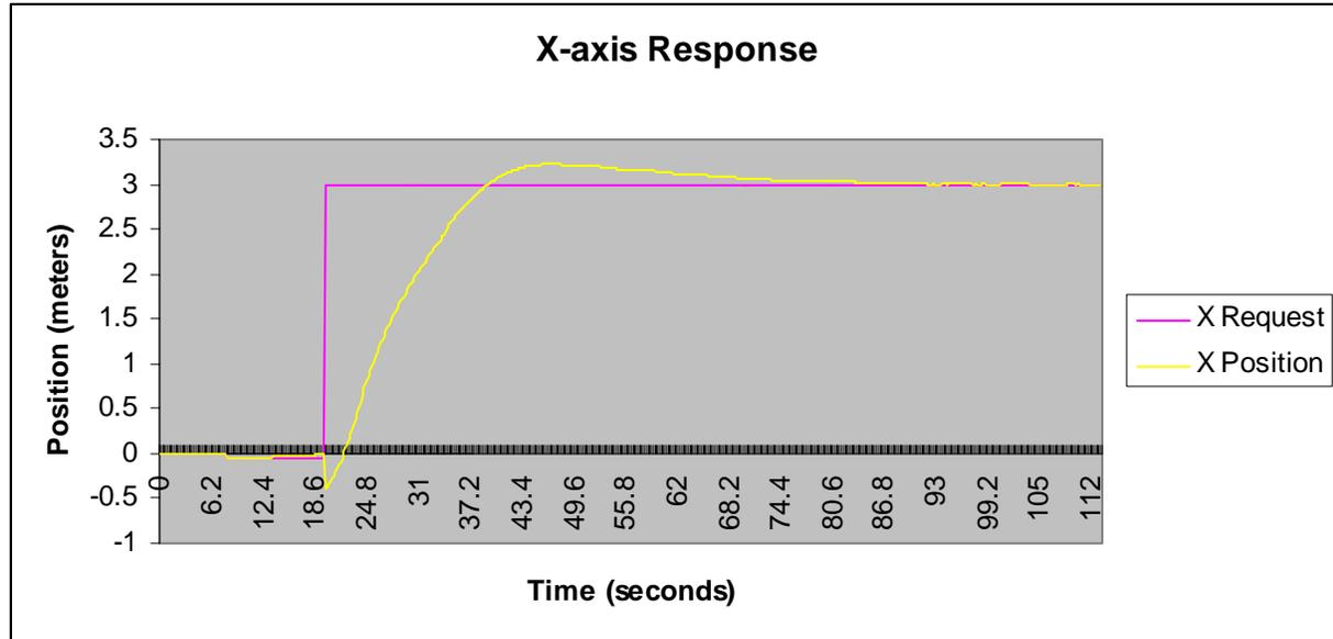
Figure 2: Typical Response to a request to a new position.
