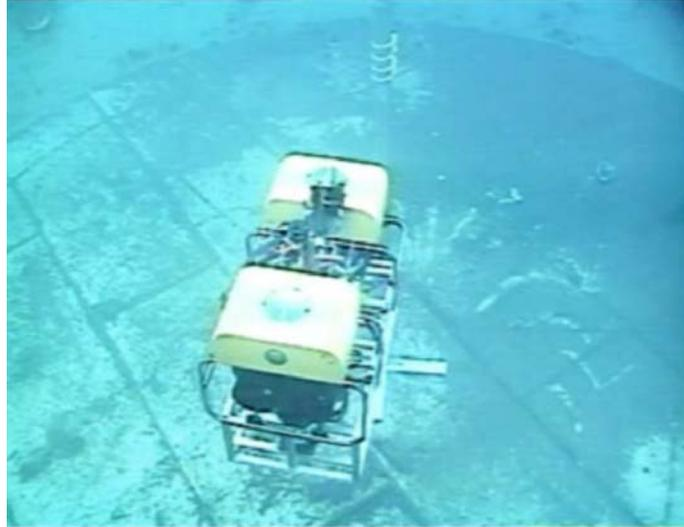
Figure 4: Automatic orbiting around a vertical target
