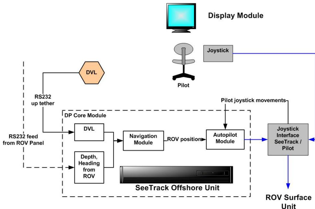
Figure 1: SeeTrack Offshore Architecture
