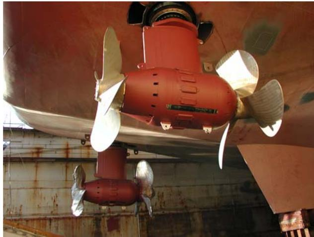
**Figure 2** Steerprop 35 CRP installed in a ROV vessel
