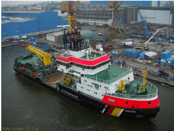
sister ship of the "NEUWERK" which is fitted with ducted mechanical thrusters and operates in the Northern Sea. Those two vessels have the same ice class and similar operational areas which gave a good chance to make a comparison between both systems. Actually aside from the well known difference in normal operations between mechanical thrusters and podded drives we found not much difference which was caused by the ice
