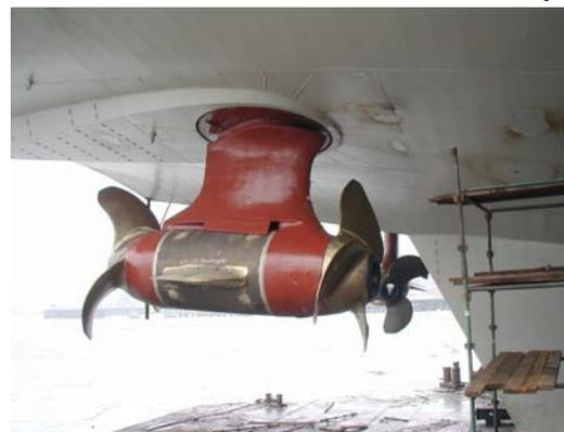
**Schottel SEP2 in an ice braking vessel** can in general be higher than with a comparable mechanical thruster.
