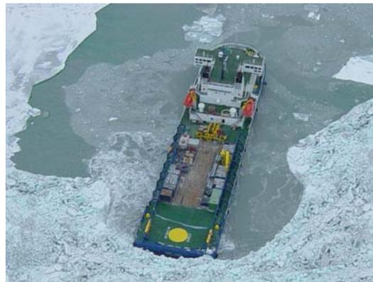
The picture on the right shows an ice class 1A super classified shallow water supply vessel during ice milling operation in the Caspian Sea.
