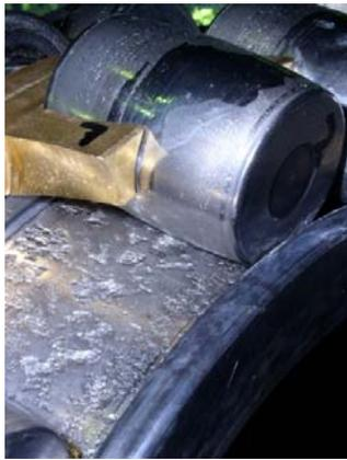
Figure 2.3. Damaged raceway, result of bad lubrication
