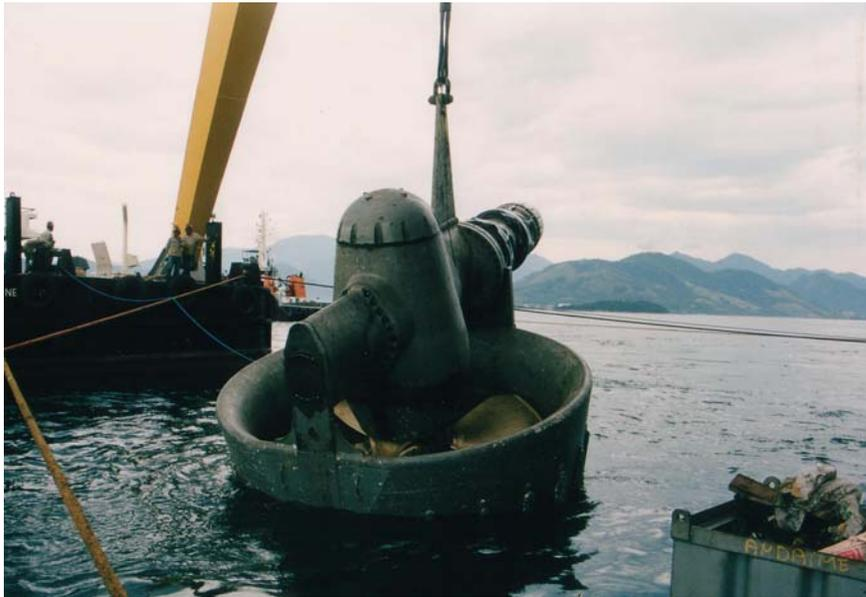
Figure 1.2. Underwater (de) mountable steerable thruster.
