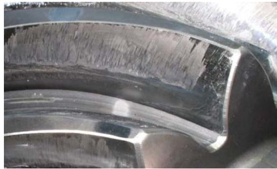
Figure 2.4. Gear mesh showing wear
