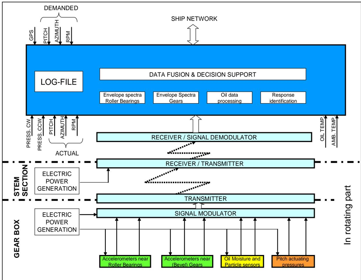
Figure 3.2. Structure of steerable thruster Health Monitoring system.
