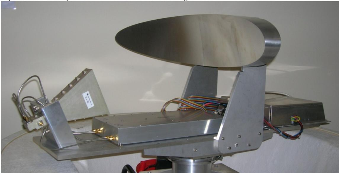
Figure 1: The RadaScan sensor with radome cover removed
