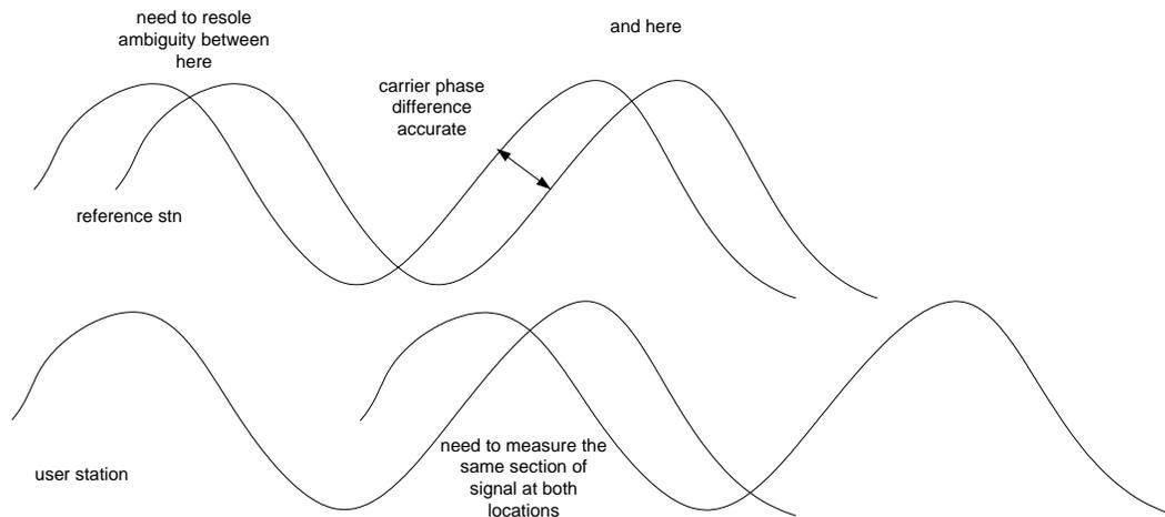
**Figure 5 Real Time Kinematic Phase Errors**
