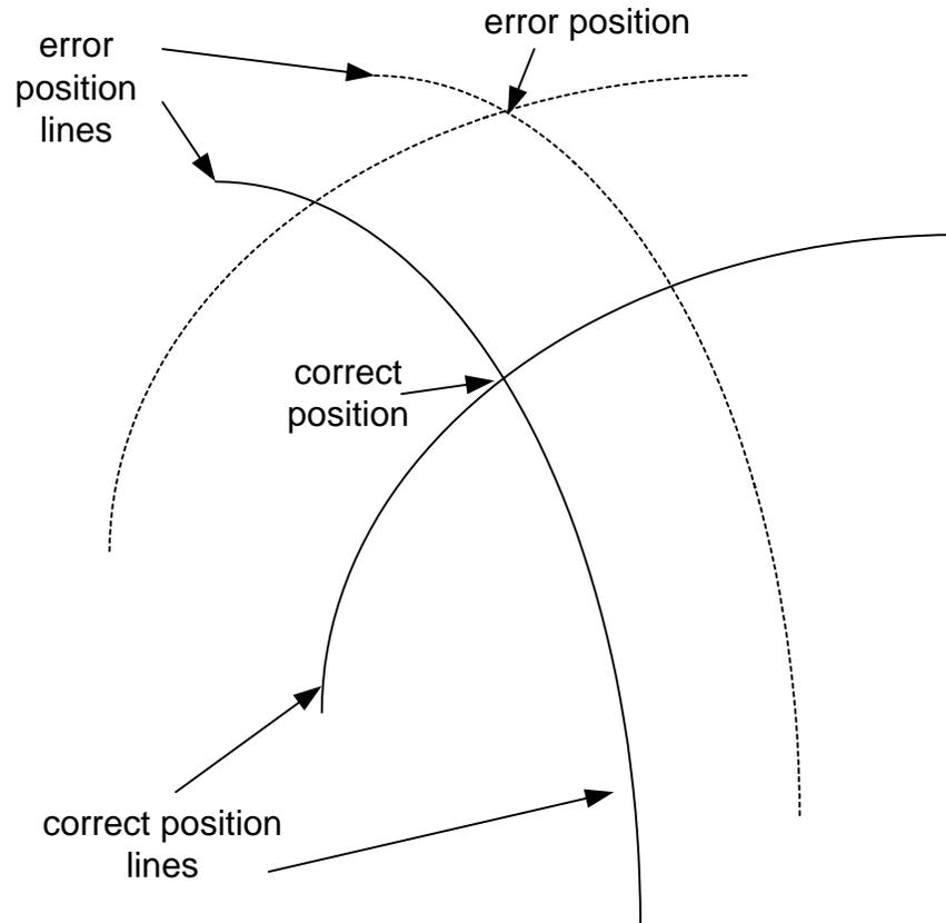
**Figure 12 Error caused by receiver clock errors**
